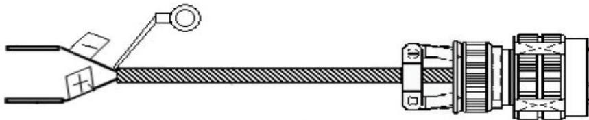
Connect one end of Military Grade power connector to the monitor, and the other end connector to the power source.
