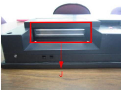
**Figure 2.4 PCI/PCIE expansion slot**
