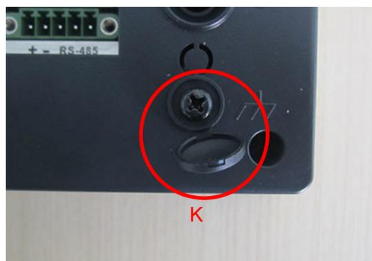
**Figure 2.5 Grounding screw**
