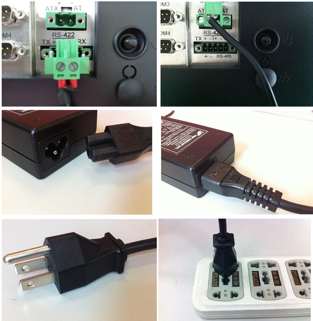
Figure 2.6 Connecting the power cable
