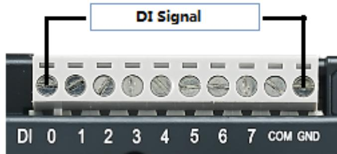
Figure 3.3 Digital Input Wiring
