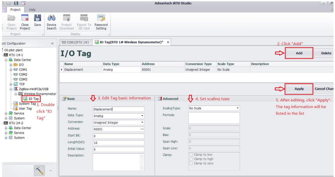
**Figure 4.14 ZigBee Meter I/O Configuration**
