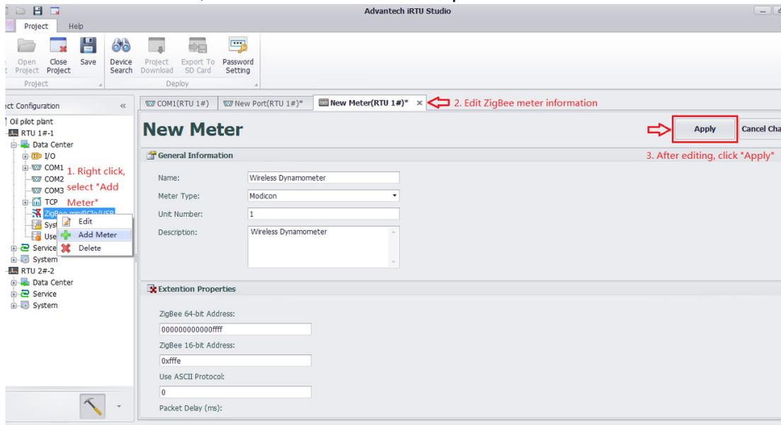
**Figure 4.13 Adding a ZigBee Meter**
