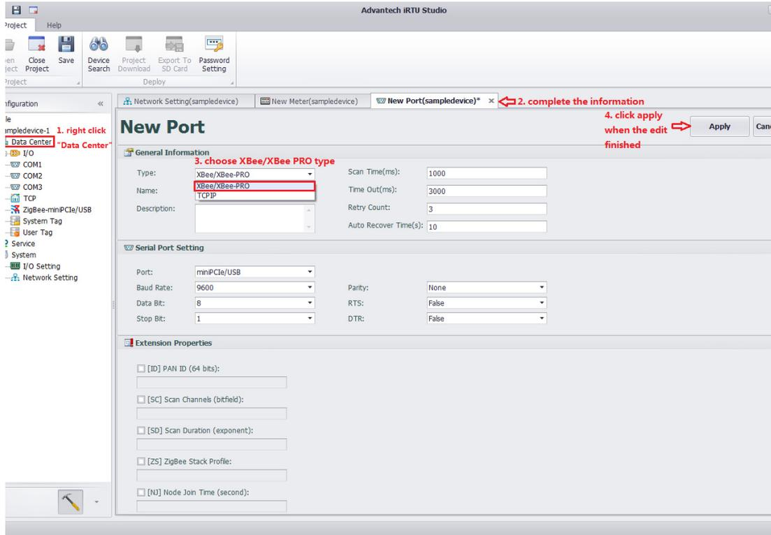
**Figure 4.12 Adding a New ZigBee Port**
