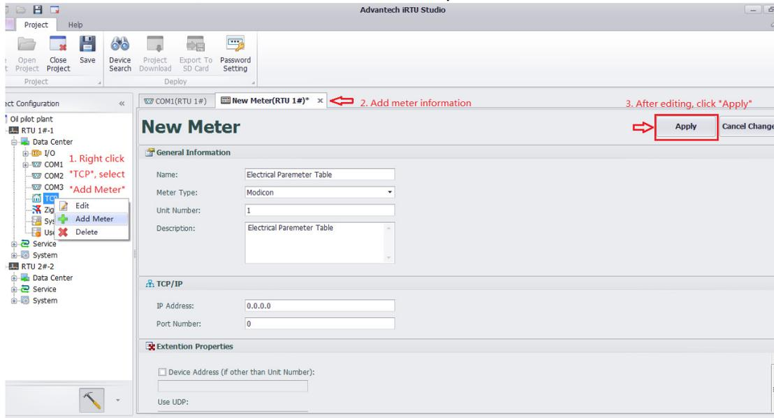
**Figure 4.9 Adding and Deleting a TCP Meter**
