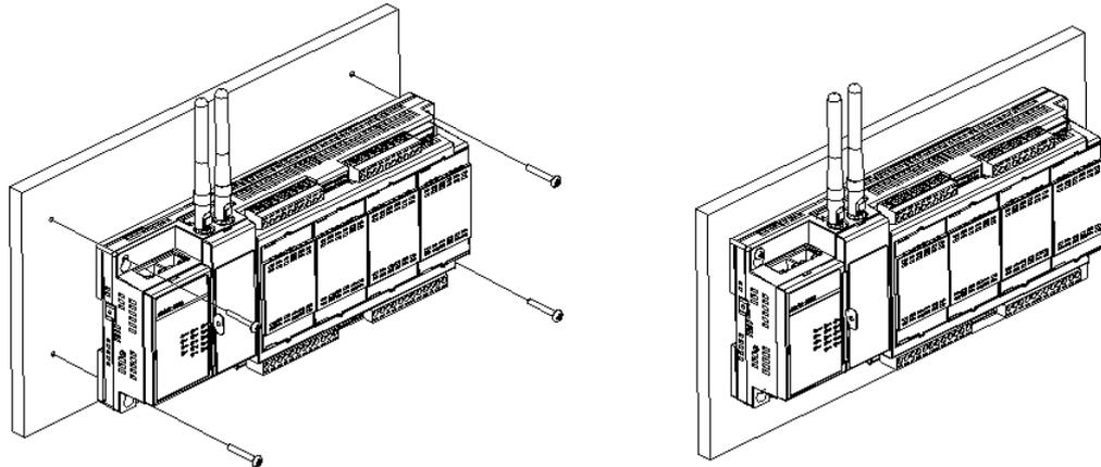
**Figure 3.6 Wall-mounted Installation**
