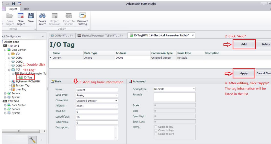
**Figure 4.10 Configuring a TCP Meters I/O**
