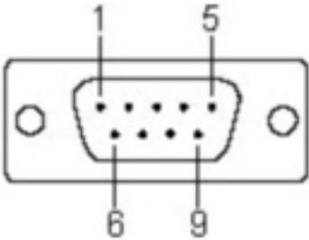
The diagram shows a top-down view of a DB-9 connector. It is a rectangular component with a central 9-pin D-sub connector. The pins are arranged in two rows: five pins in the top row and four pins in the bottom row. Four specific pins are labeled with numbers: pin 1 is the top-left pin, pin 5 is the top-right pin, pin 6 is the bottom-left pin, and pin 9 is the bottom-right pin. There are two circular mounting holes on the left and right sides of the connector housing.
