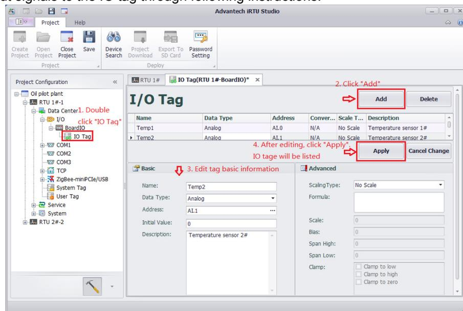
Figure 4.5 Configuring Onboard I/O
