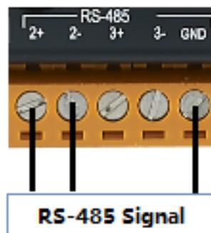
Figure 3.5 Serial Port Wiring
