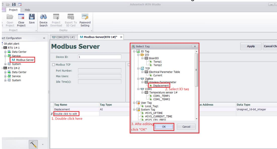
Figure 4.16 Adding I/O Tags to the Modbus Address List
