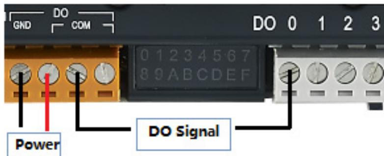
Figure 3.4 Digital Output Wiring
