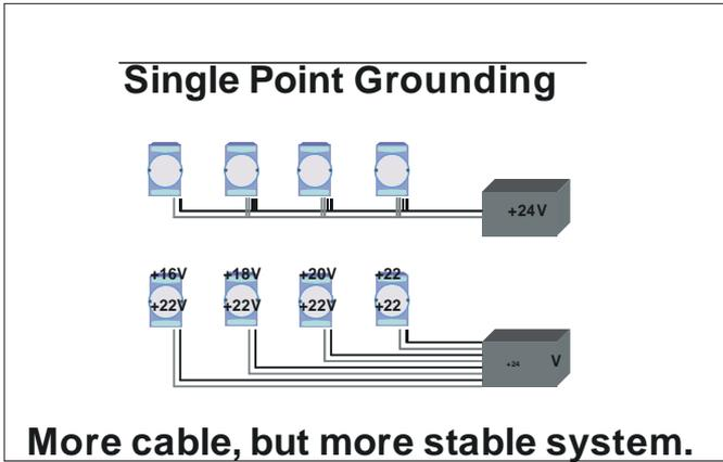
*Figure F-8 : Single point ground in F.(2)*
