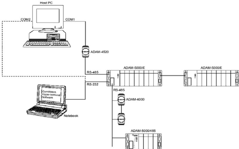
*Figure 2-8 Build-in Communication Ports for Diagnostic Connection*
