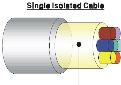
Use **Aluminum foil** to cover those wires, for isolating the external noise.
