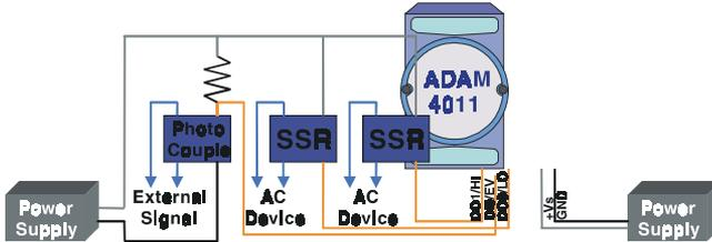
**Separate Load and Device power.**
