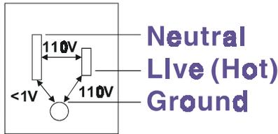
**Normal Mode:** refers to defects occurring between the live and neutral conductors.
