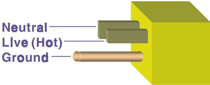
Ground-pin is longer than others, for first contact to power system and noise bypass.
