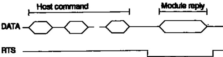
*Figure C-7 RS-485 data flow control with RTS*
