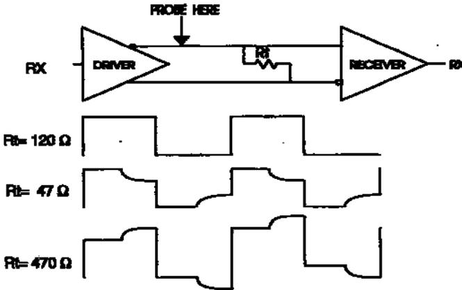
*Figure C-5 Signal distortion*
