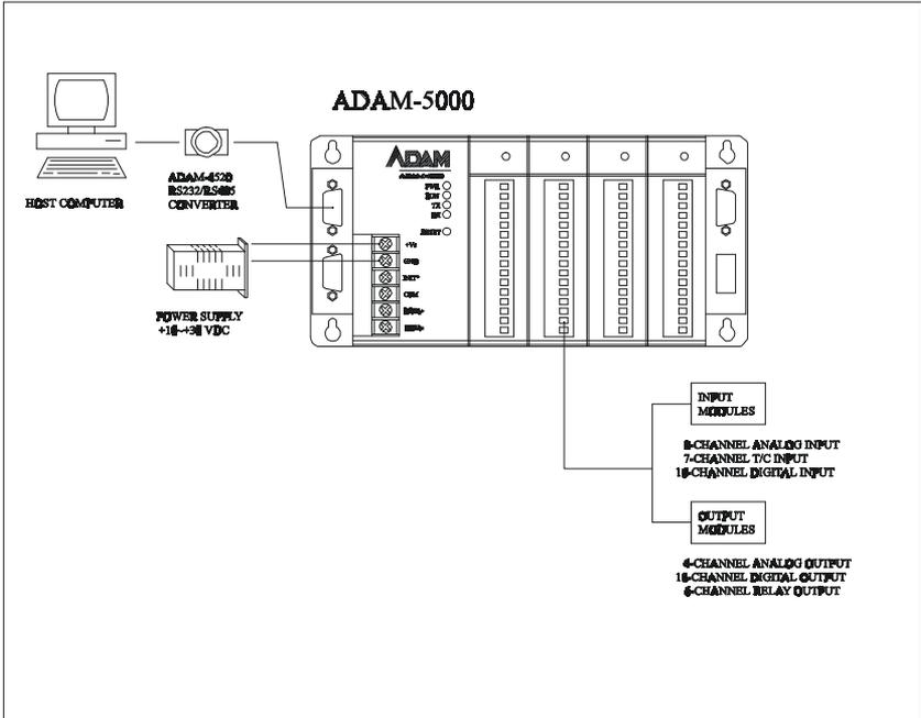
**Note:** To avoid system over heating, only four ADAM-5024 are allowed to be installed on ADAM-5000E.
