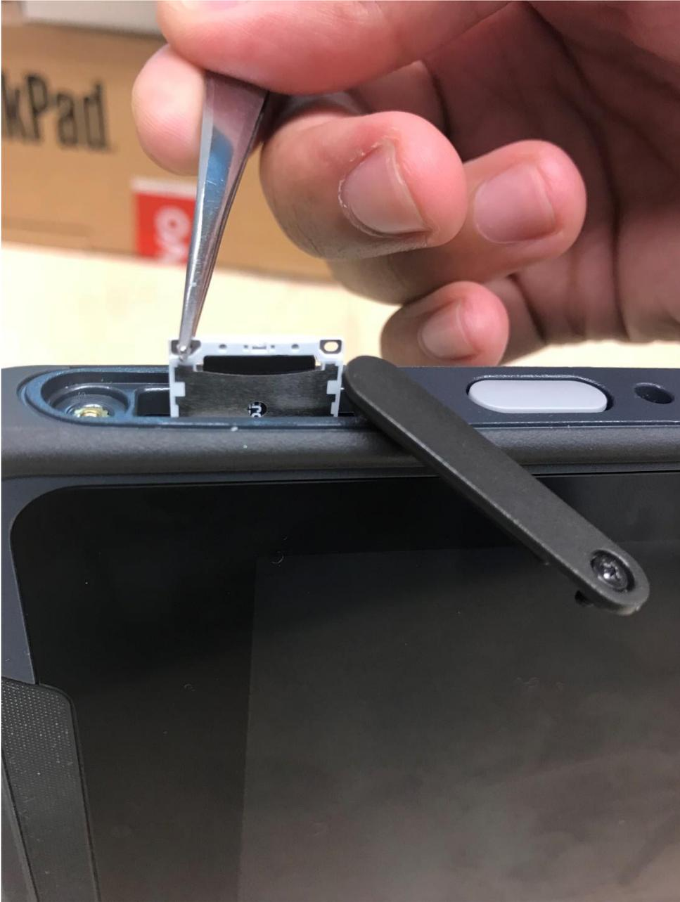
**Step4:** Put the SIM card and Micro SD card on the card tray and push it into same place.
