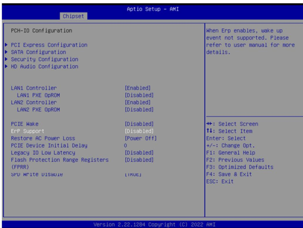
When ErP is enabled, restore AC power loss & the below features are not supported.
