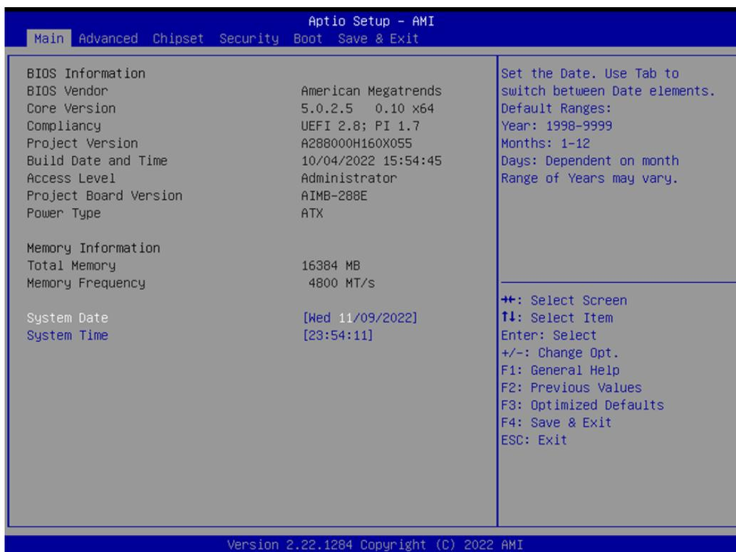
The Main BIOS setup screen has two main frames. The left frame displays all the options that can be configured. Grayed-out options cannot be configured; options in blue can. The right frame displays the legend.
