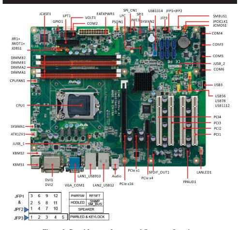
Figure 1: Board Layout: Jumper and Connector Locations
