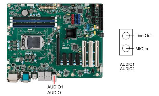
Line Out can be connected to external audio devices like speakers or headphones. Mic In can be connected to a microphone.
