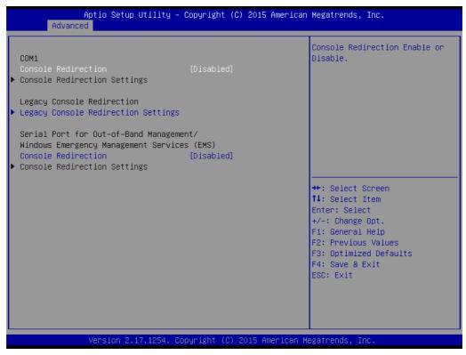
Figure 3.24 Serial Port Console Redirection
