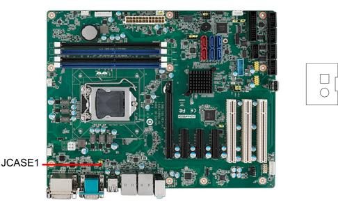
JCASE1 is for chassis with a case open sensor. The buzzer on the motherboard sounds if the case is opened unexpectedly.
