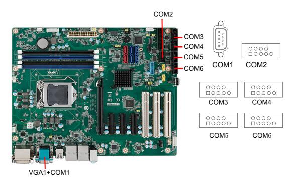
The AIMB-785 offers six serial ports (one on the rear panel and five onboard). RS-232/422/485 mode is selected by BIOS for COM3. These ports can connect to a serial mouse, printer or communications network. The IRQ and address ranges for
