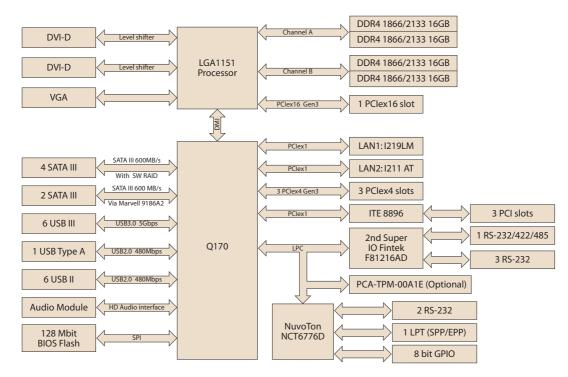
Figure 1.3 AIMB-785 Block Diagram
