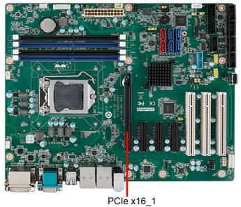
The AIMB-785 provides a PCIe x16 slot for users to install an add-on peripheral card for extension requirements.
