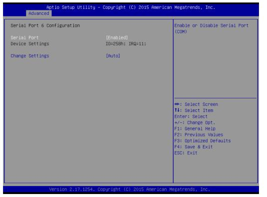
Figure 3.23 Serial Port 6 Configuration
