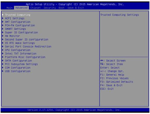
Figure 3.3 Advanced BIOS features setup screen
