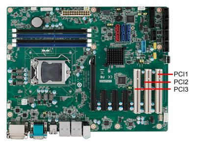
The AIMB-785 provides four 32-bit / 33 MHz PCI slots.
