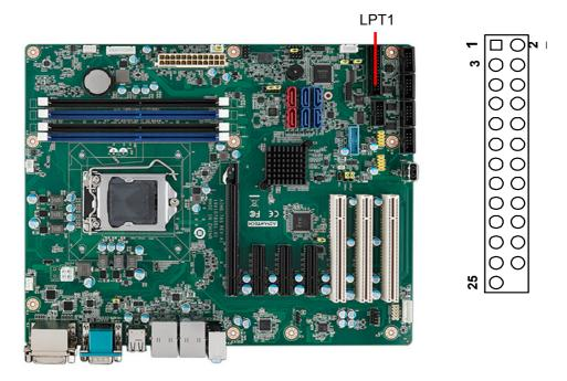
The parallel port is normally used to connect the motherboard to a printer. The AIMB-785 includes an onboard parallel port, accessed through a 25-pin flat-cable connector, LPT1.
