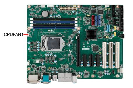
If a fan is used, this connector supports cooling fans that draw up to 500 mA (6 W).
