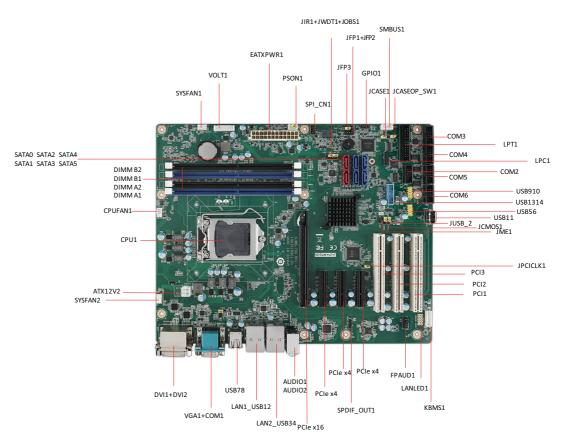
Figure 1.1 Jumper and Connector Locations
