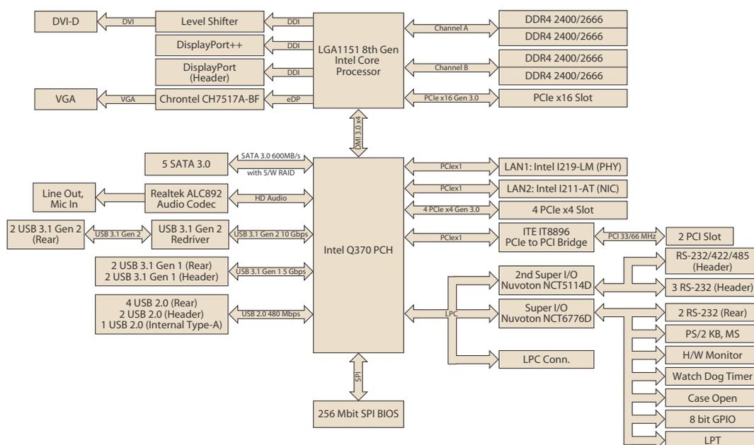
Figure 1.3 Block Diagram
