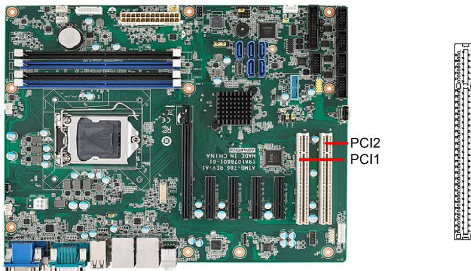
The AIMB-786 provides two 32-bit / 33 MHz PCI slots.
