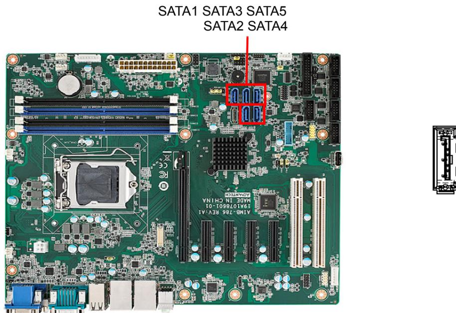
AIMB-786 features five high performance serial ATA 3.0 interfaces (up to 600 MB/s) with long, thin, easy-to-run SATA cables.
