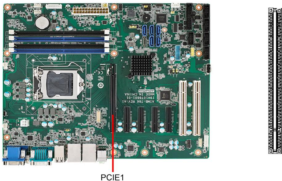
The AIMB-786 provides a PCIe x16 slot for users to install an add-on peripheral card for extension requirements.
