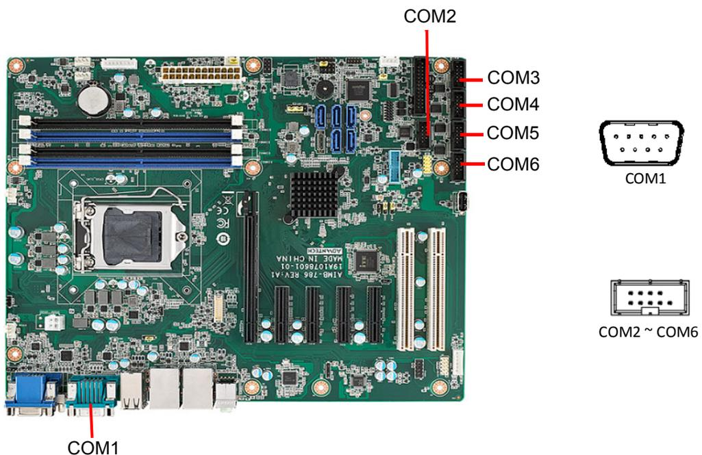
The AIMB-786 offers six serial ports (one on the rear panel and five onboard). COM3 can be configured as RS-232/422/485 by jumper settings (see Chapter 1), and selecting correct device mode for RS-485 under BIOS is necessary (see Chapter 3). These ports can connect to a serial mouse, printer or communications network. The IRQ and address ranges for those ports are fixed. However, if you want to disable the port or change these parameters later, you can do this in the system BIOS setup. Dif-
