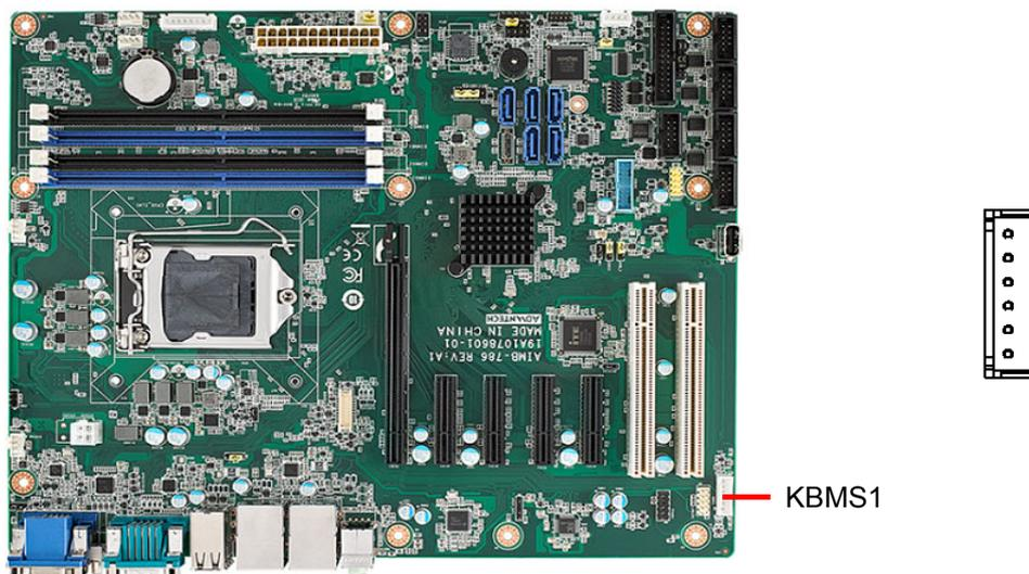
A 6-pin header on the motherboard is for an optional PS/2 keyboard/mouse cable. This gives system integrators greater flexibility in designing their systems.
