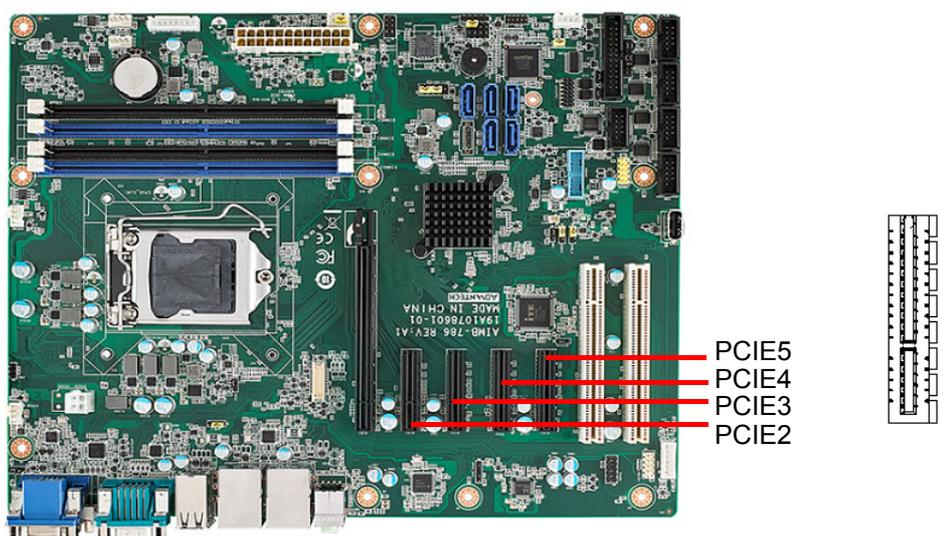
The AIMB-786 offers four PCIe x4 slots for users to install add-on cards for extension requirements.
