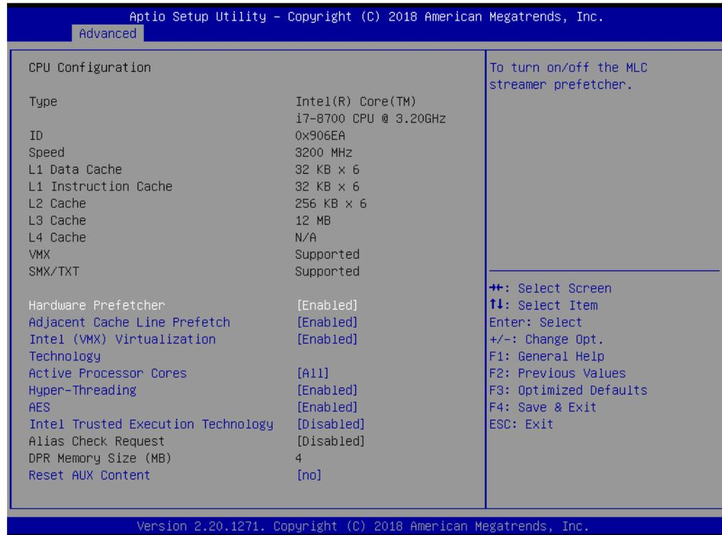
Figure 3.5 CPU Configuration
