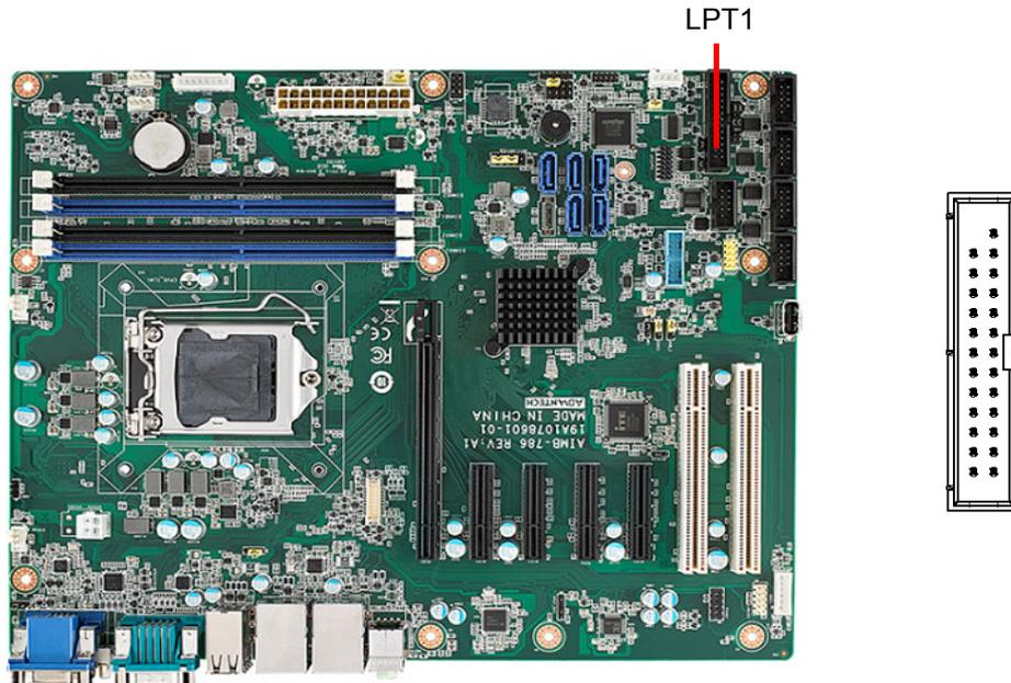
The parallel port is normally used to connect the motherboard to a printer. The AIMB-786 includes an onboard parallel port, accessed through a 25-pin flat-cable connector, LPT1.
