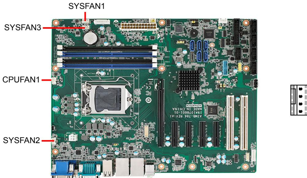
If a fan is used, this connector supports cooling fans that draw up to 500 mA (6 W).
