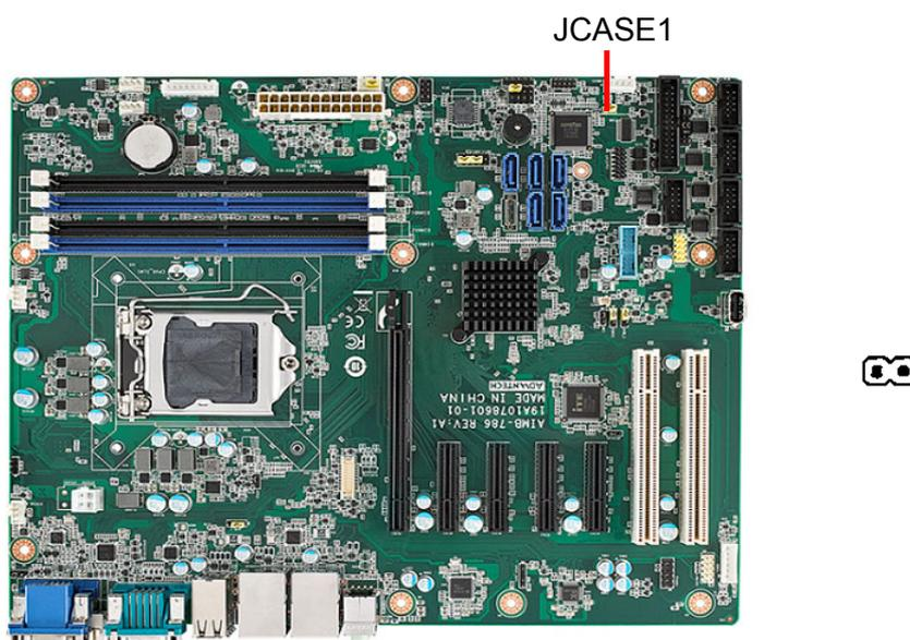
JCASE1 is for chassis with a case open sensor. The buzzer on the motherboard sounds if the case is opened unexpectedly. The default function is disabled and pins 1-2 is bridged by a jumper cap.
