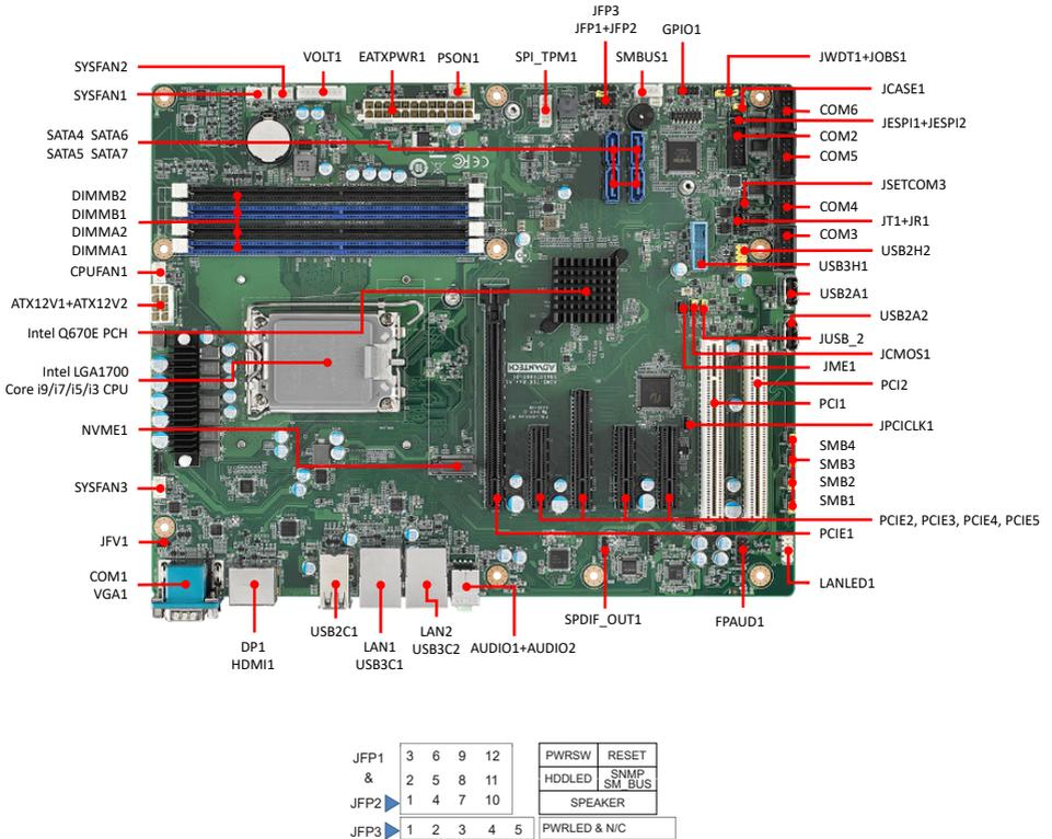
Figure 1: Board Layout: Jumper and Connector Locations
