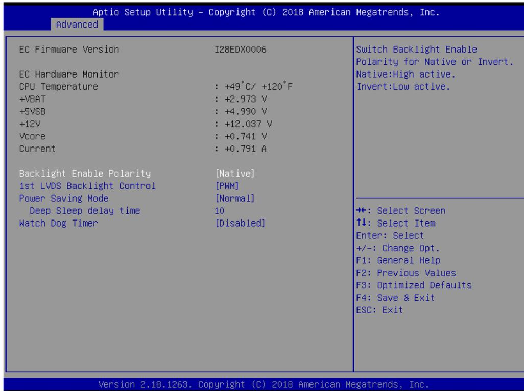
Embedded controller configuration displays all information about system Temperature/Voltage.
