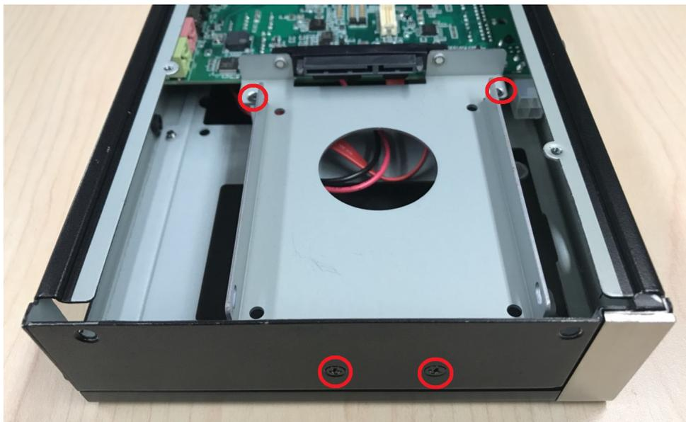
3. Install the HDD/SSD into the HDD bay, and fix the HDD onto the bracket.
