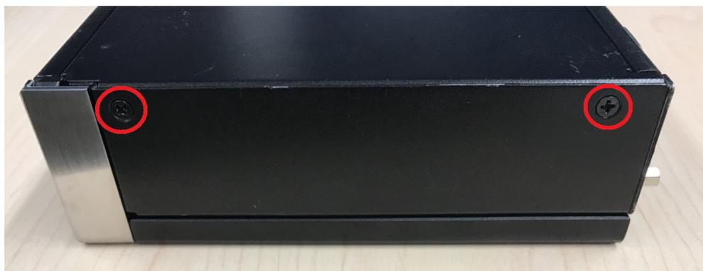
2. Unscrew the 4 screws on the HDD bay.
