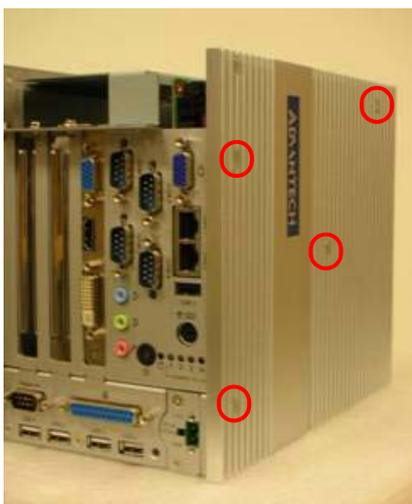
Figure 2.23 Unscrew 4 screws and remove the right side cover
