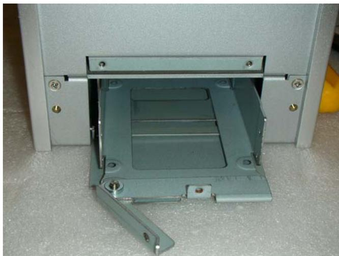
**Figure 2.15 Pull out the HDD bracket**
