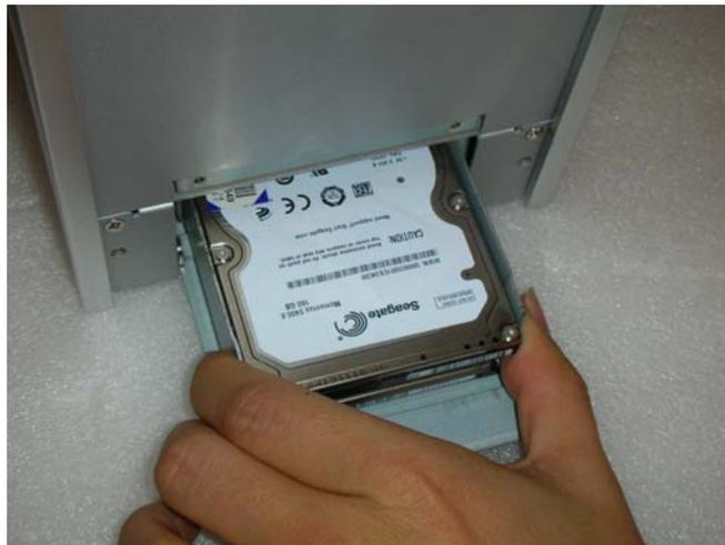
**Figure 2.17 Insert the bracket into the HDD housing**
