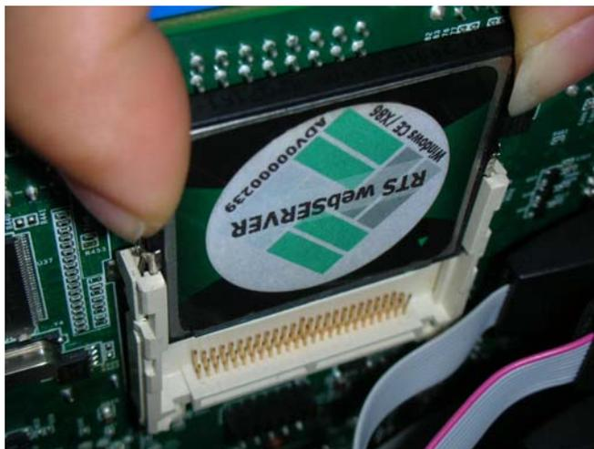
**Figure 2.21 Install the CF card**
