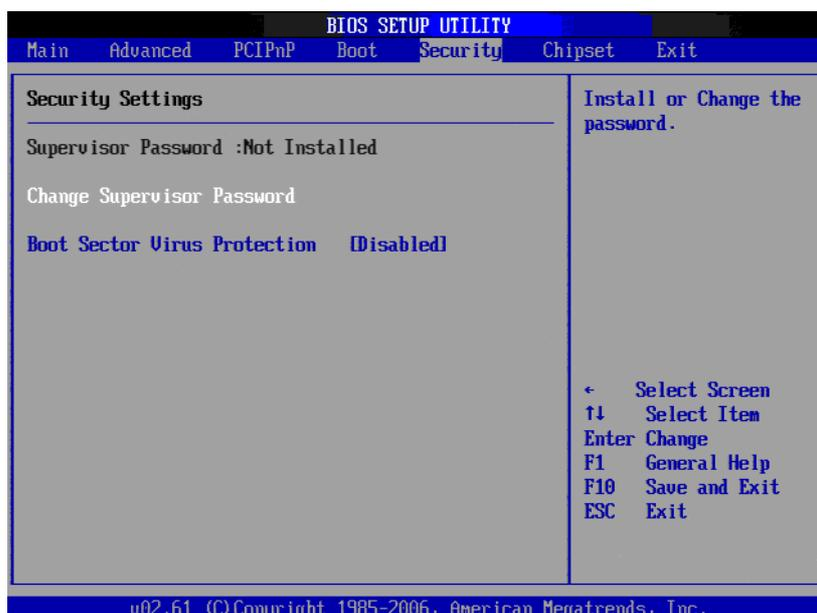
**Figure 3.14 Password Configuration**
