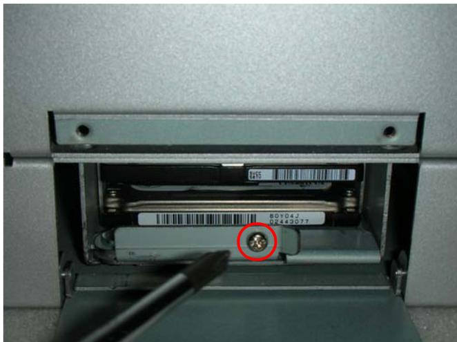
Figure 2.18 Secure the HDD housing with screw
