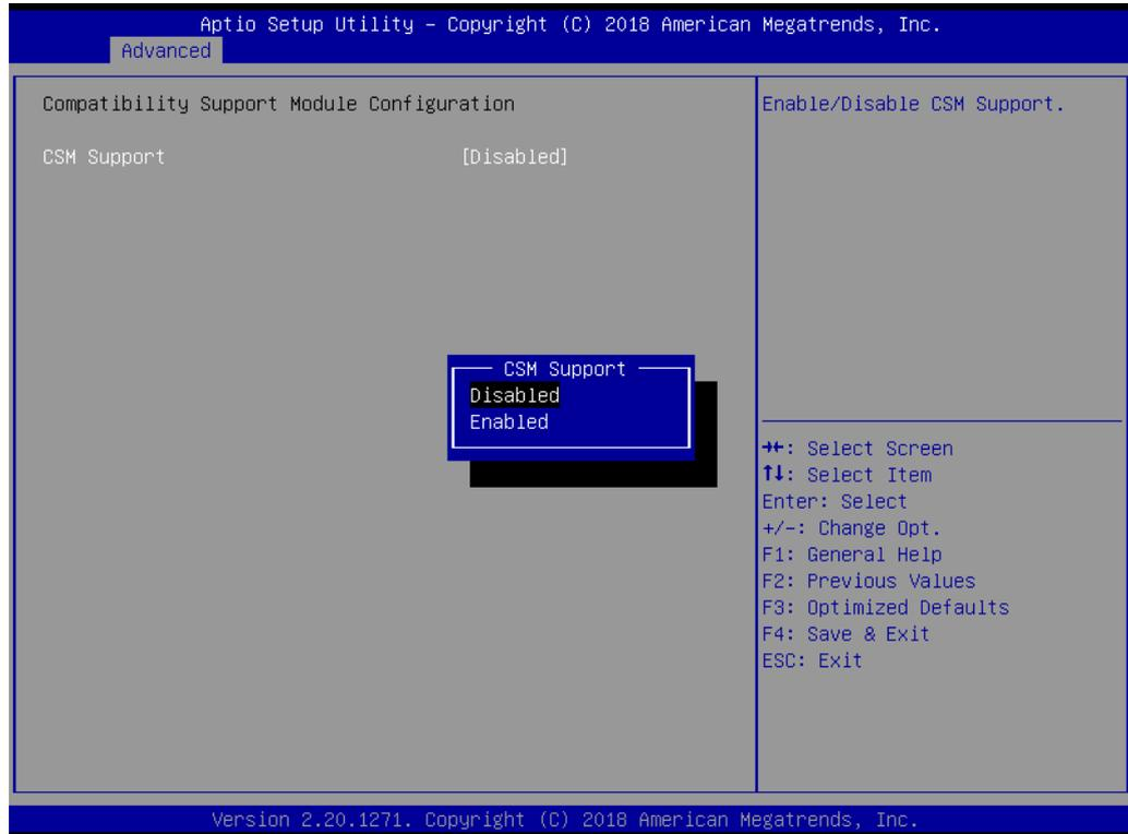
**Figure 3.20 CSM configuration screen**
