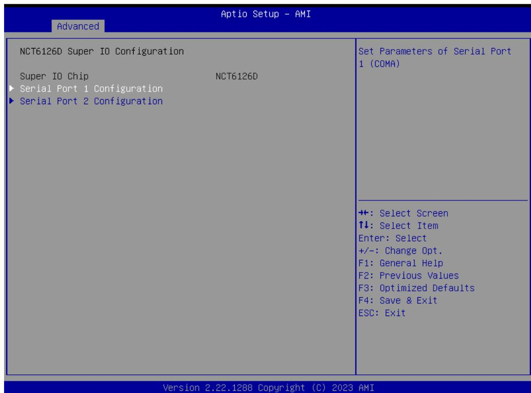
Figure 3.18 NCT6126D Super IO Configuration
