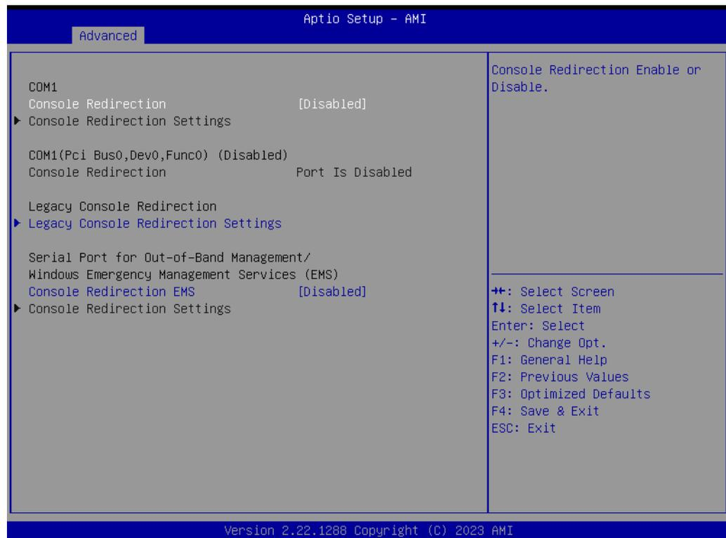
**Figure 3.23 Serial Port Console Redirection**
