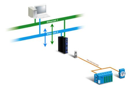
**Figure 2.1 Dual Ethernet Connections**
