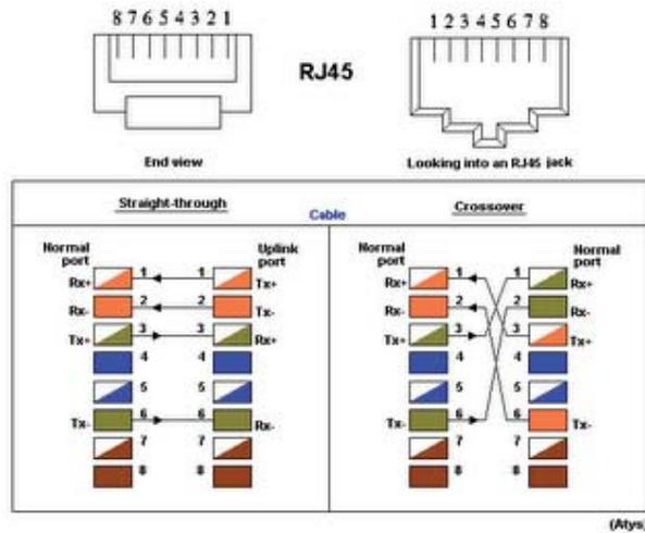
Figure 3.2 VDSL Interface Pin Assignments (RJ-45)
