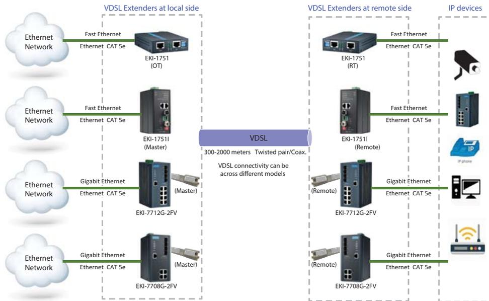
Figure 1.2 Deployment Option (Point to Point)
