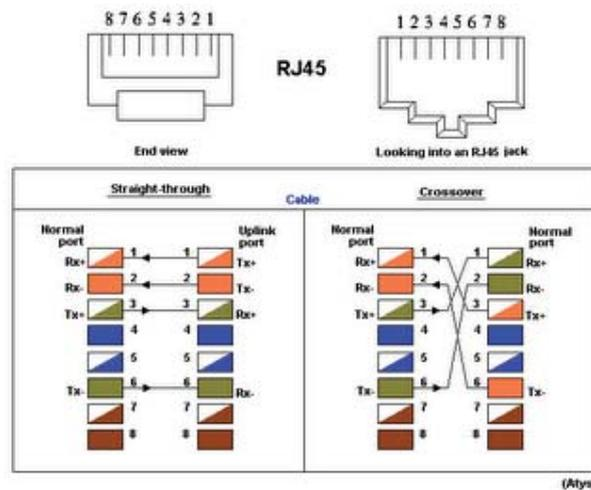
Figure 3.1 Ethernet Port Connector (RJ-45)
