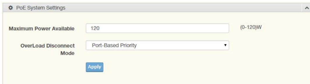
Figure 4.113 Management > Power Over Ethernet > PoE System Settings
