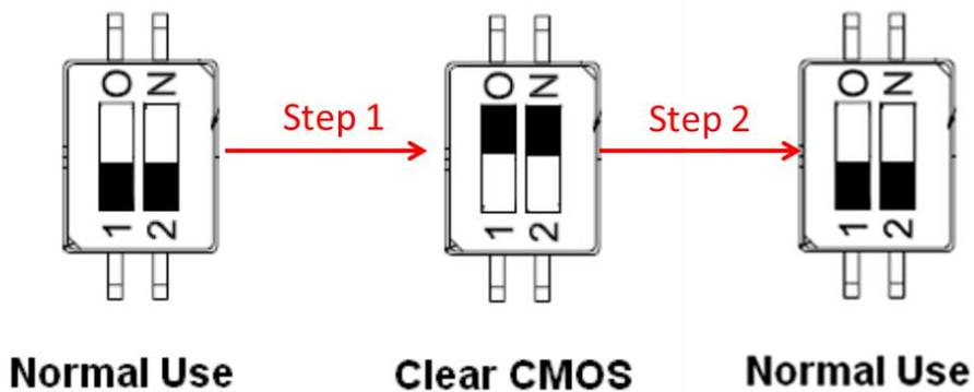
**Step 1:** To set the jumper to “clear” position, switch 1 to 0, 2 to N.
