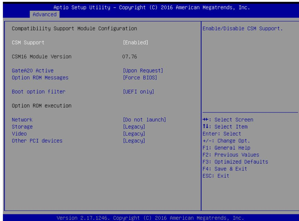
Figure 2.13 CSM configuration
