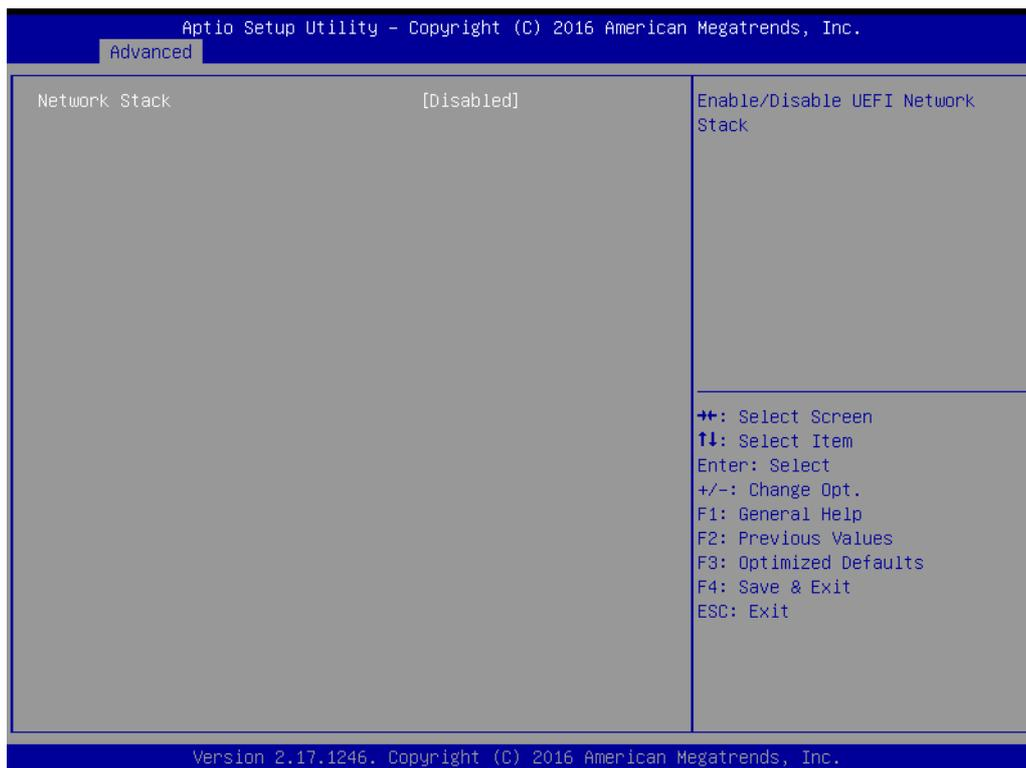
**Figure 2.12 Network Stack configuration**
