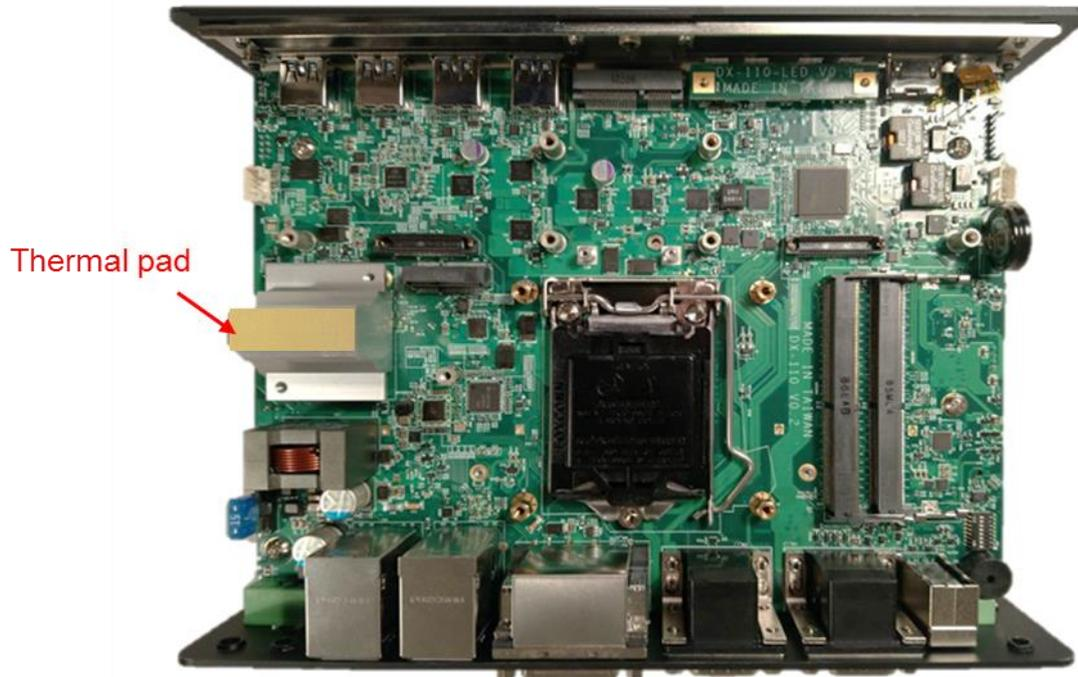
**Note: Before assembling the system's chassis cover, please make sure the protective film on the Thermal Pad has been removed!**
