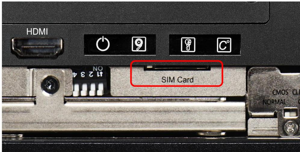
2. Insert a SIM card into SIM slot with the gold contacts facing up. Please pay attention to the insert orientation as illustrated.
