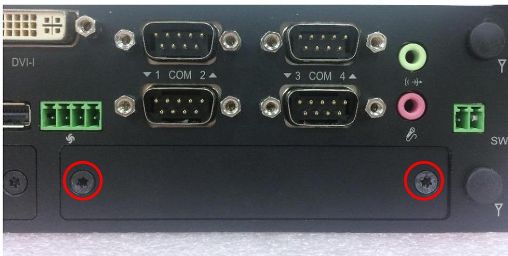
3. Insert the CMI-DIO module carefully into the CMI connector on main board. Fix it with 2 screws.
