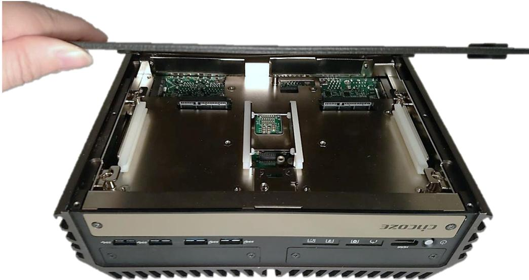
2. Fasten the bottom cover with 6 screws.
