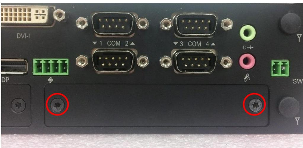
3. Insert the CMI-COM module carefully into the CMI connector on main board. Fix it with 2 screws.
