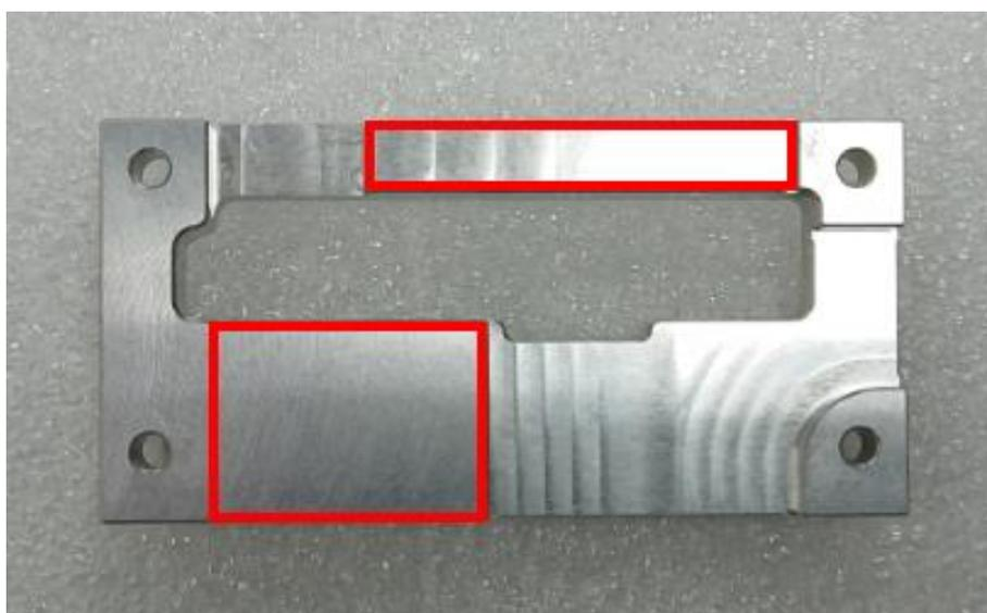
5. Paste two thermal pads for CFM-PoE01 onto the heatsink carefully.
