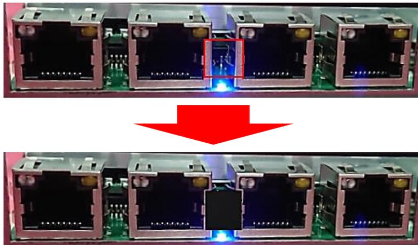
2. Insert the CMI-LAN module for DX-1100 vertically to the female connector (BTB\_FH2 or BTB\_FH4) on system's mainboard until it is connected firmly, and fasten 4 copper pillars to fix it. (CMI-M12LAN module is taken as the installation example in this chapter)
