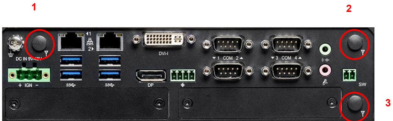
2. For antenna 1 and antenna 2, please penetrate the antenna jack through the hole at both sides as illustrated.
