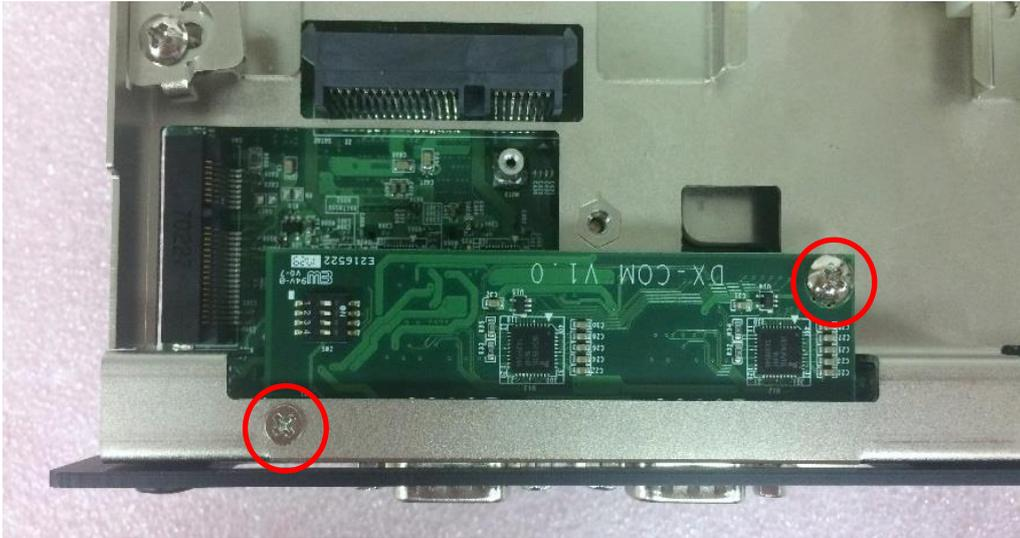
4. Loosen the 4 D-Sub jack screws as marked on photo.
