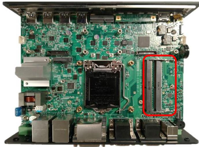
2. Insert a SO-DIMM at a 45-degree angle until its edge connector is connected to SO-DIMM socket firmly.
