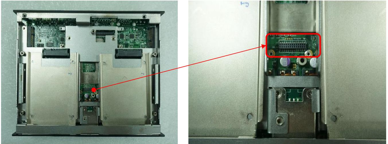
2. Fasten 1 copper pillar before insert IGN module.
