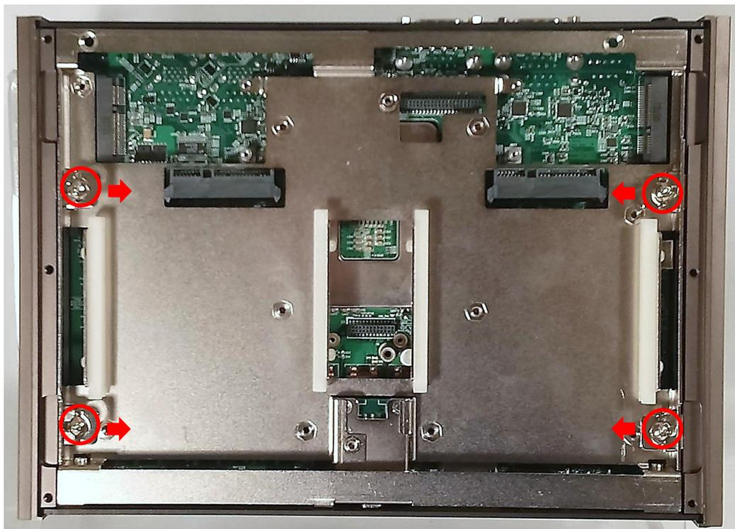
4. Hold front and rear panel and lift up the body of unit vertically.
