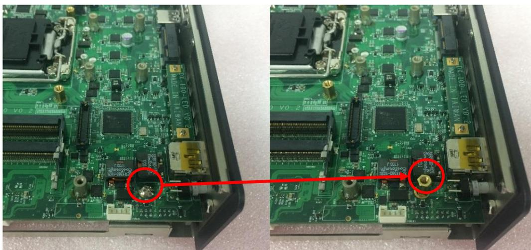
5. Insert the CMI module vertically into the female connector on system's mainboard until it's connected firmly and fasten 4 screws to fix it.
