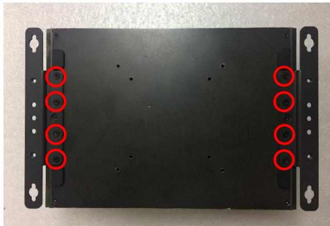
2. There are 2 bracket mounting holes at left and right side for customer fix the system on the wall.
