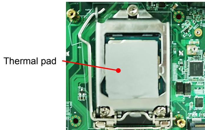
**Note: Before putting on the thermal block (in the next step), please make sure the protective film on the Thermal Pad has been removed!**
