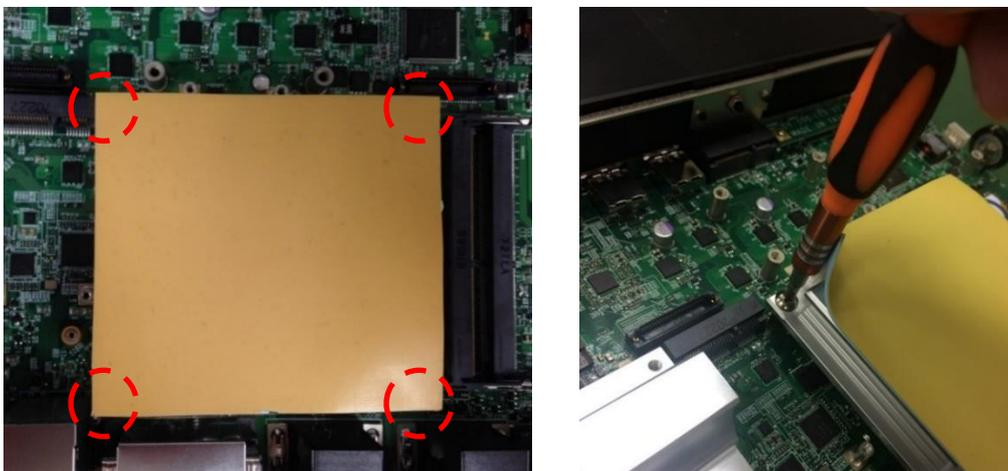
**Note: Before assembling the system's chassis cover, please make sure the protective film on the Thermal Pad has been removed!**
