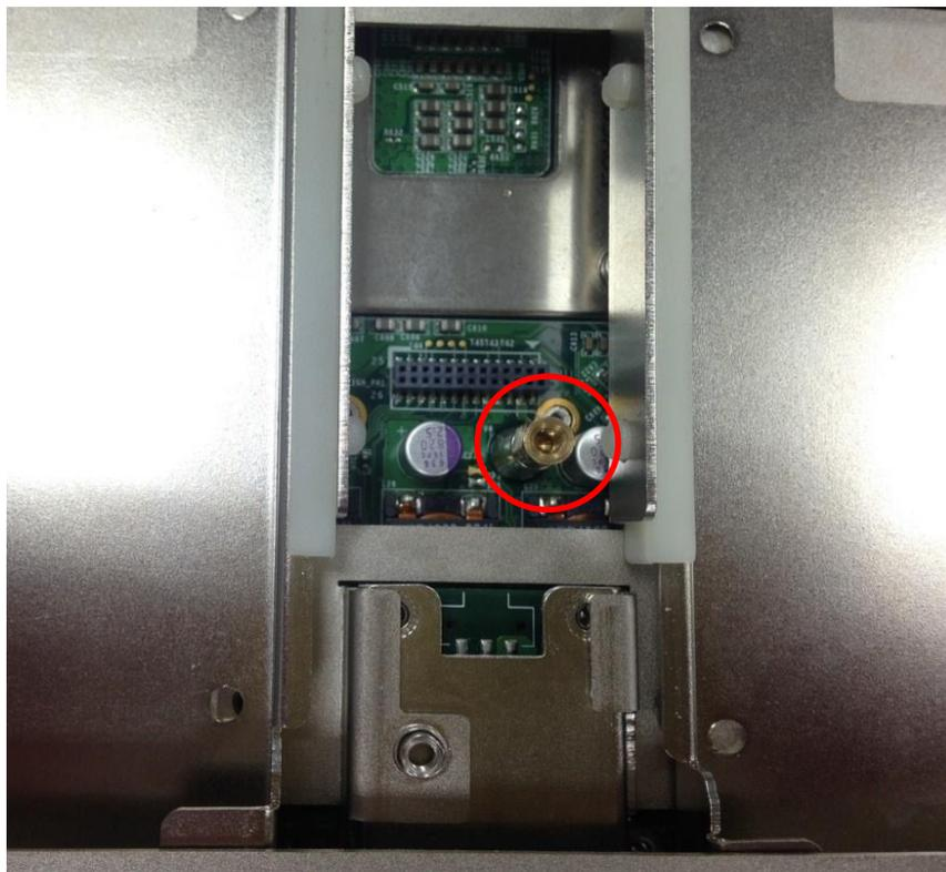
3. Insert IGN module vertically to the female connector on the system's mainboard, and fasten 2 screws to fix it.
