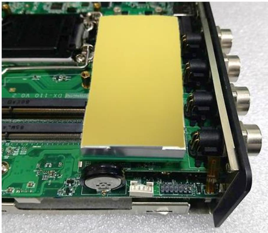
**Note: Before assembling the system's chassis cover, please make sure the protective film on the Thermal Pad has been removed!**
