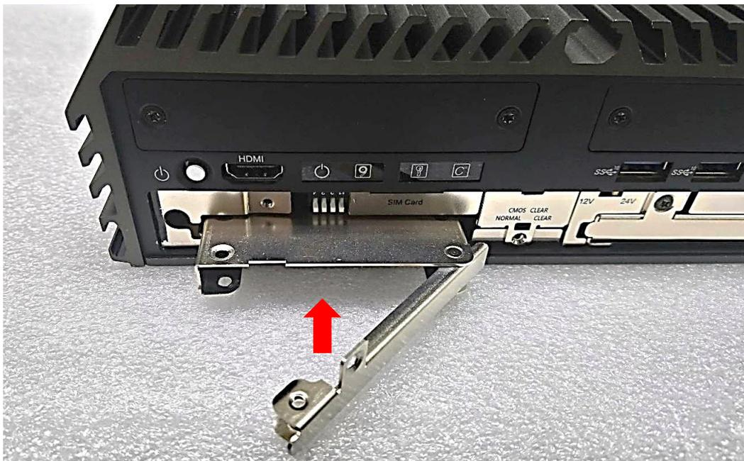
5. Place the rotating arm back and fasten the screw.
