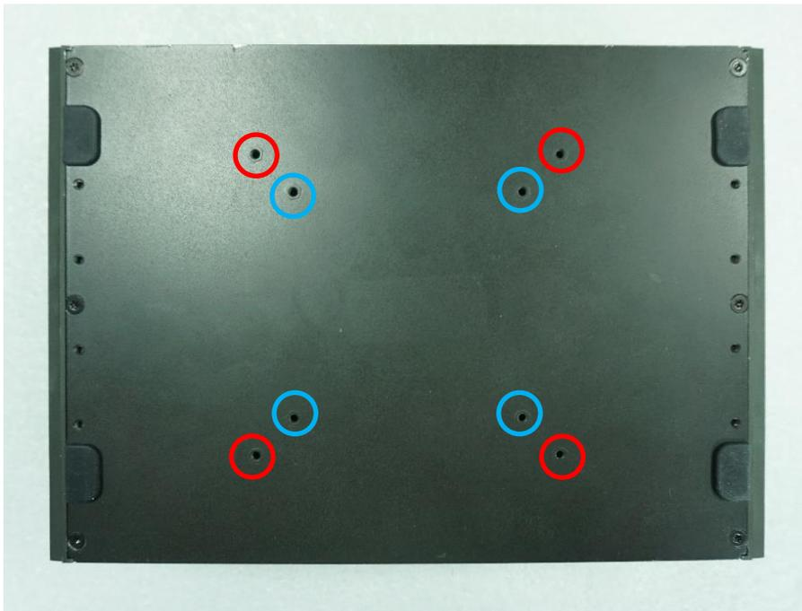
1. The following picture illustrates the installation of DX-1100 series on a VESA stand. Align the 4 screw holes of VESA stand with the screw holes on bottom side of system. Fasten 4 screws to fix it.
