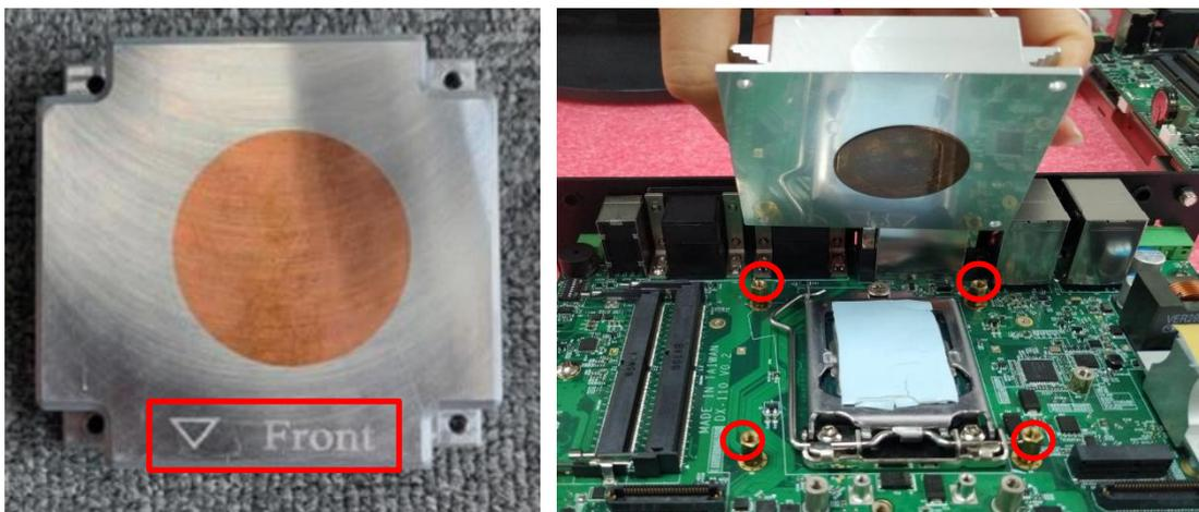
7. Flip the corner of thermal pad and fasten the heatsink with provided 4 screws.
