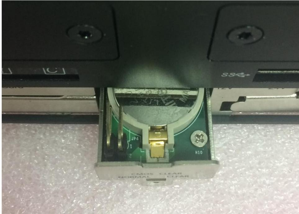
3. Insert a CMOS battery in the battery slot.
