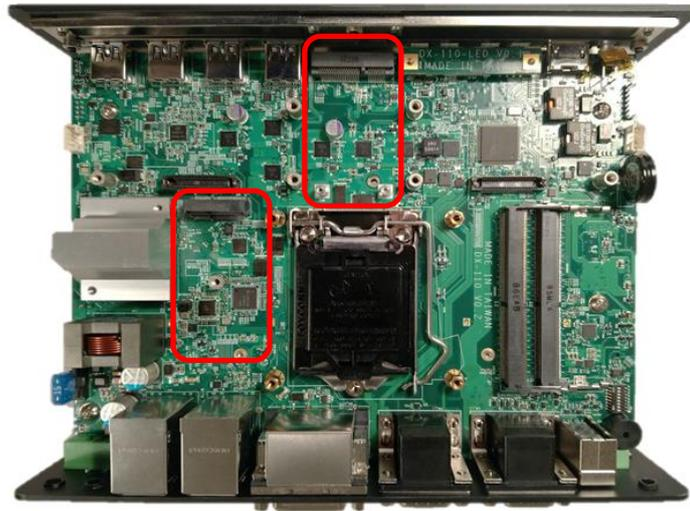
2. Insert the Mini-PCIe card at a 45-degree angle until its edge connector is connected firmly into slot. For 3G/4G Mini-PCIe card, please install onto CN3 slot.
