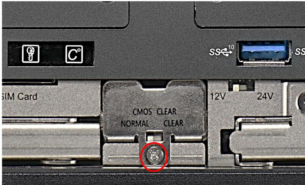
2. Pull out the CMOS battery bracket with assistance of a tweezer.
