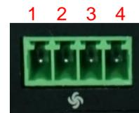
**COM1 / COM2 / COM3 / COM4: RS232 / RS422 / RS485 Connector**
