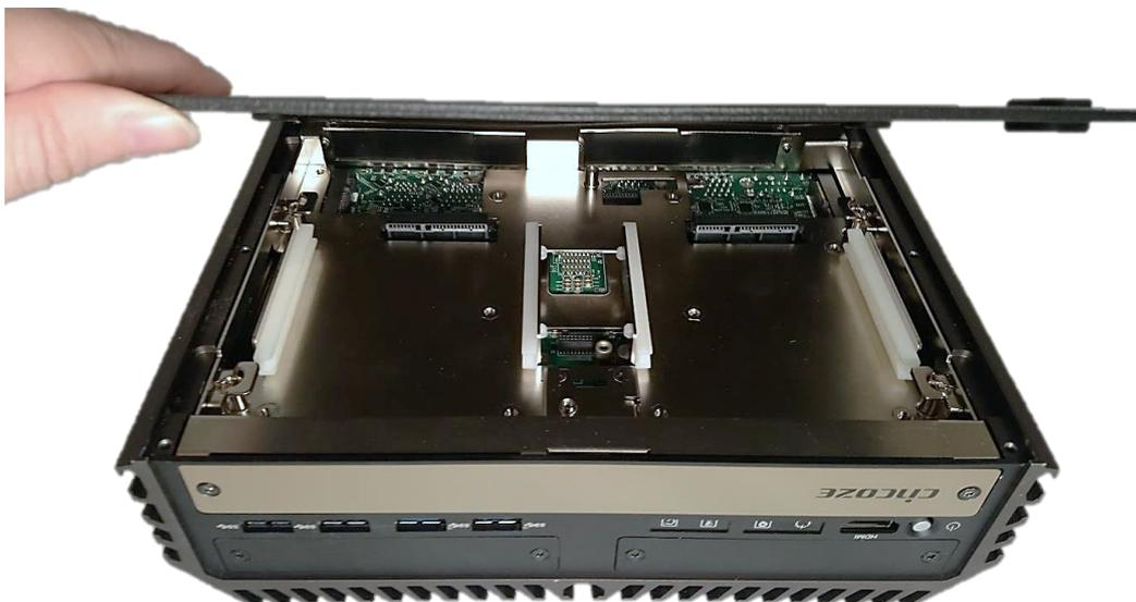
3. Loosen the 4 screws. Pull out 4 latches as marked on photo.
