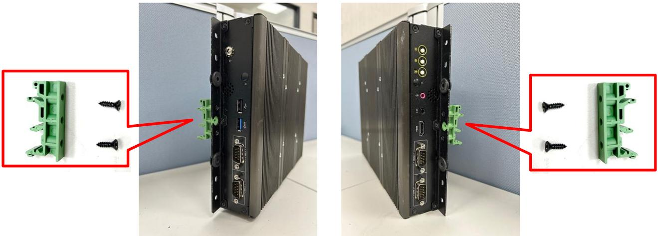
Step 3. Clip the system into DIN rail as illustrated by the following steps. (1) Have upper end of mounting clip snaps into the DIN rail. (2) Press the system toward to have lower end of mounting clip snaps into the other side of DIN rail.
