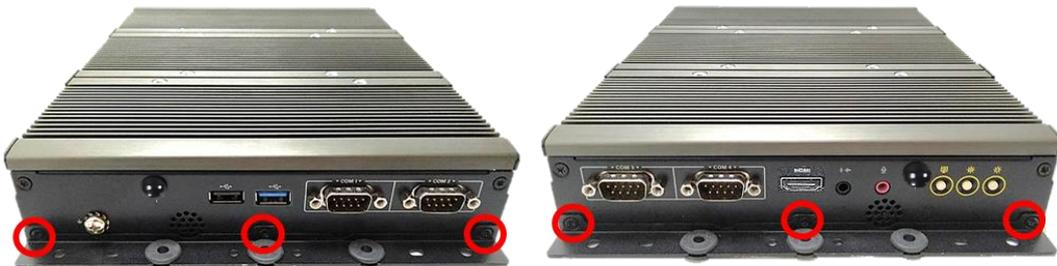
Step 4. Attach the P2202 to wall by fastening screws through mounting holes at each side as illustrated.
