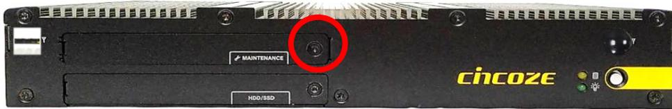
Step 2. Locate the SIM card slot.
