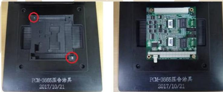
2. Put your board on PCM SBC board and align the two connectors, and then press the red handle of fixture.
