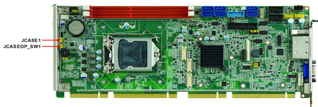
Figure 2.2 PCE-5128/7128 Case Open Jumper Locations
