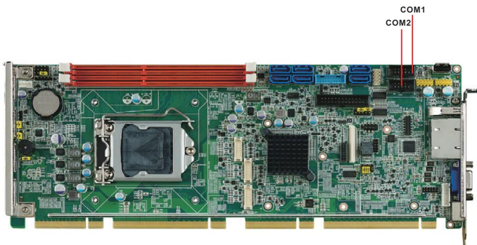
The PCE-5128/7128 offers two serial ports. These ports can connect to serial devices, such as a mouse or a printer, or to a communications network.
