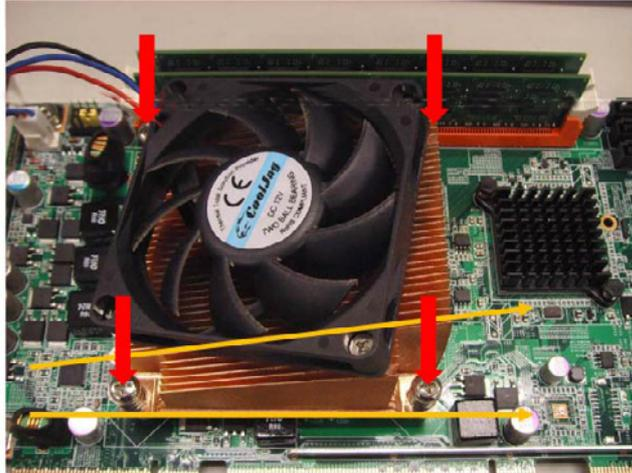
Note the direction of CPU cooler; it must follow that shown above. Installing a CPU cooler in the wrong direction may cause poor heat dissipation that may damage the CPU card.
