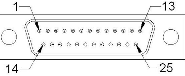
The diagram shows a top-down view of a male DB25 connector. It has a rectangular shape with two rows of pins: a top row of 13 pins and a bottom row of 12 pins. Four pins are specifically labeled with arrows: pin 1 (top-left), pin 13 (top-right), pin 14 (bottom-left), and pin 25 (bottom-right). There are two circular mounting holes on the sides of the connector.
