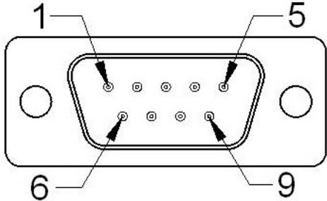
The diagram shows a top view of a male DB9 connector. It has a rectangular shape with a central row of nine pins. Four pins are specifically labeled with arrows and numbers: pin 1 is the top-left pin, pin 5 is the top-right pin, pin 6 is the bottom-left pin, and pin 9 is the bottom-right pin. There are two circular mounting holes on the left and right sides of the connector housing.
