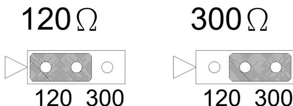
**Figure 2.23 Resistor Selection (for PCI-1602 and PCIe-1622 series)**
