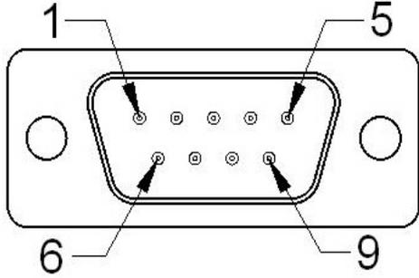
The diagram shows a top-down view of a male DB9 connector. It has a rectangular shape with a central row of nine pins. Four pins are specifically labeled with arrows: pin 1 (top-left), pin 5 (top-right), pin 6 (bottom-left), and pin 9 (bottom-right). There are two circular mounting holes on the sides of the connector.
