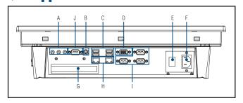
A: Line in/Line out/Mic in B: PS2 Mouse & Keyboard C: USB 2.0 x 4
