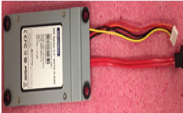
Figure 2.10 Secure SATA HDD with screws
