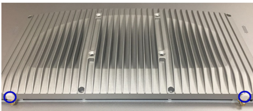
Figure 2.17 Removing plugs for the antennae
