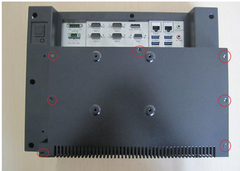
**Figure 2.22 Complete assemble expansion kits**
