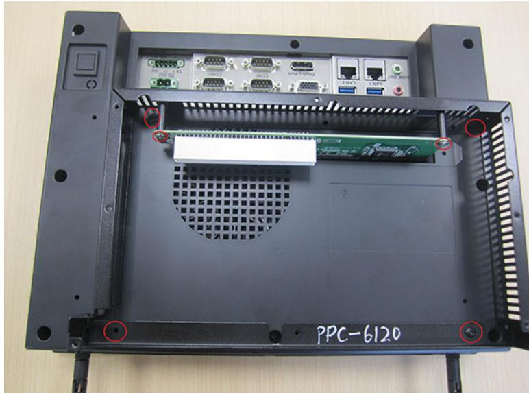
**Figure 2.21 Assemble riser card**
