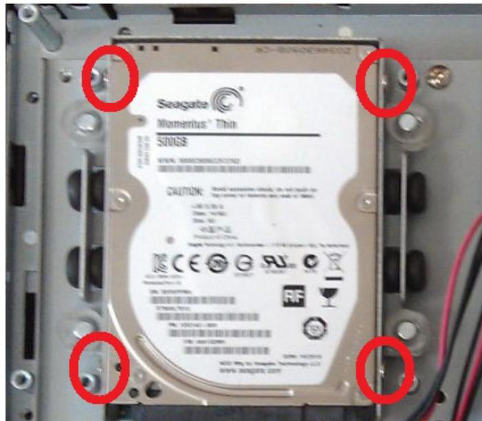
**Figure 2.13 Fix HDD in HDD brackets**
