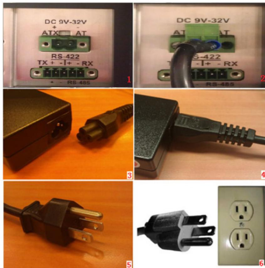
Figure 2.4 Connecting Power Cord
