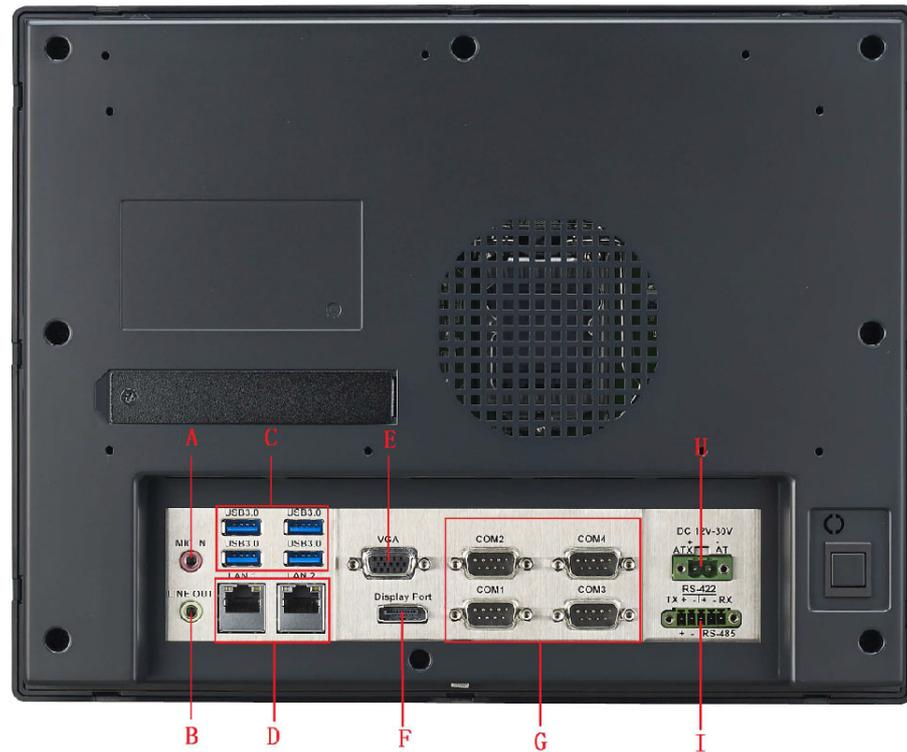
**Figure 2.3 IO Connectors of Panel PC**
