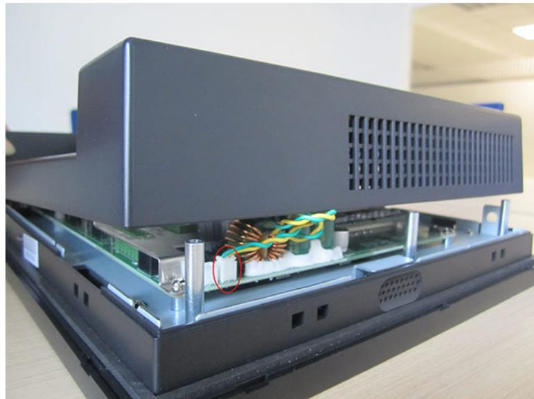
**Figure 2.6 Unplugging Switch Wire**
