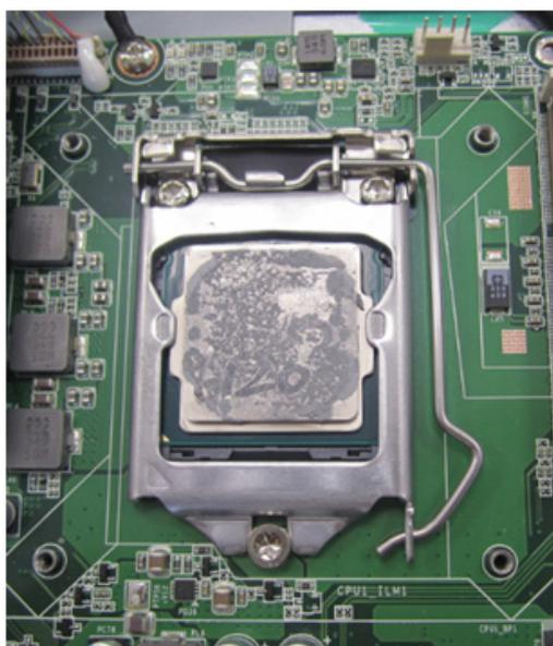
**Figure 2.8 CPU fasten in socket**
