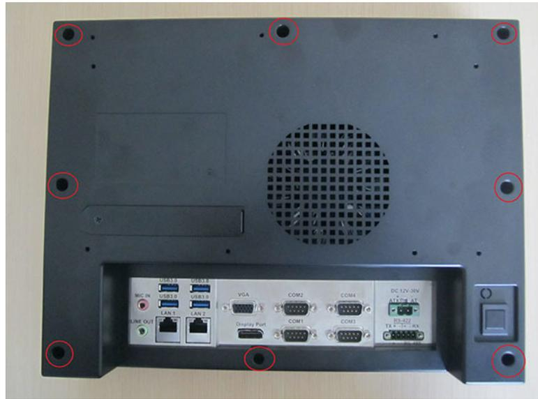
**Figure 2.5 Unfastening Screws on Rear Cover**
