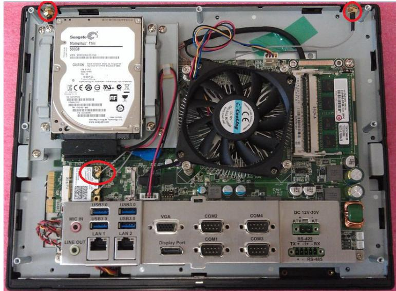
**Figure 2.17 Replace the HDD module**
