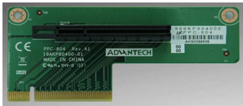
The total current load provided by PPC-8150 /PPC-8170 PCIe slot is no more than 25 W.
