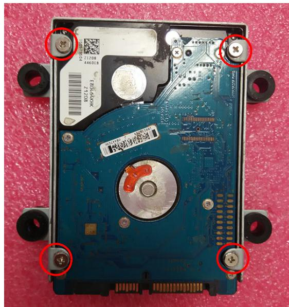
Figure 2.11 HDD Screws
