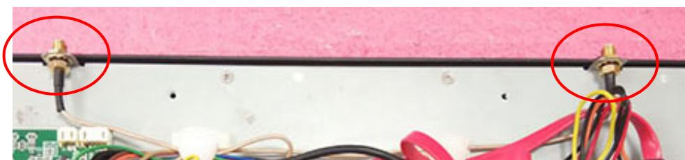
Figure 2.19 Antenna Connection
