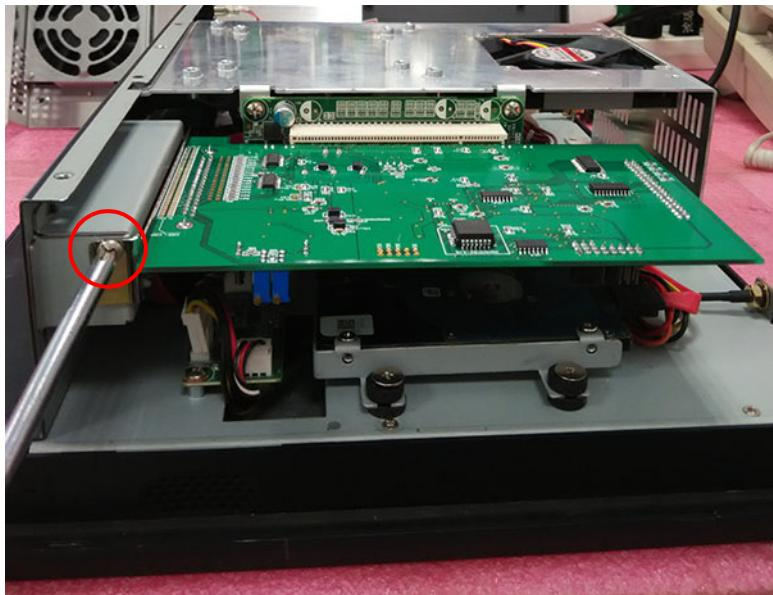
Figure 2.16 Secure PCI Card
