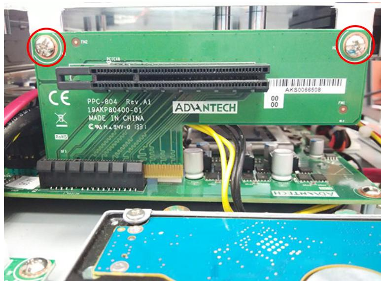
Figure 2.13 PCIe Riser card installation
