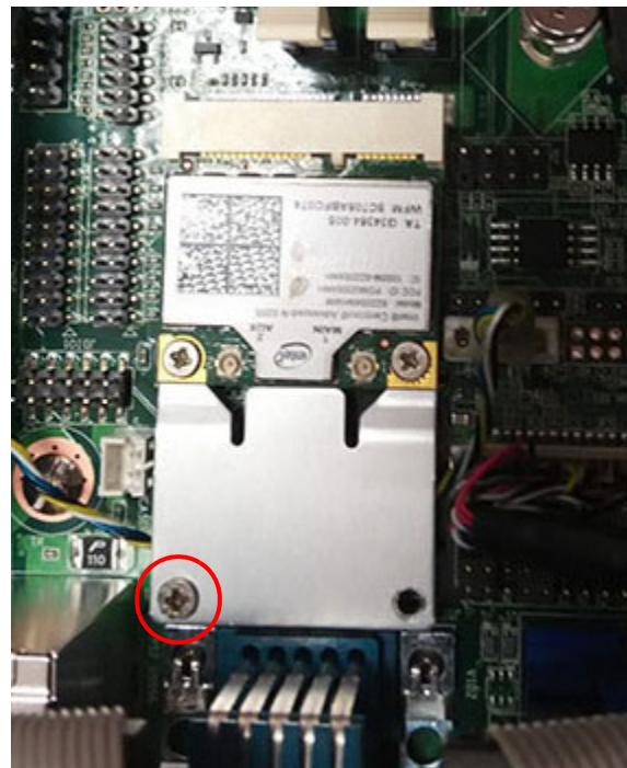
Figure 2.18 Wireless Card Installation
