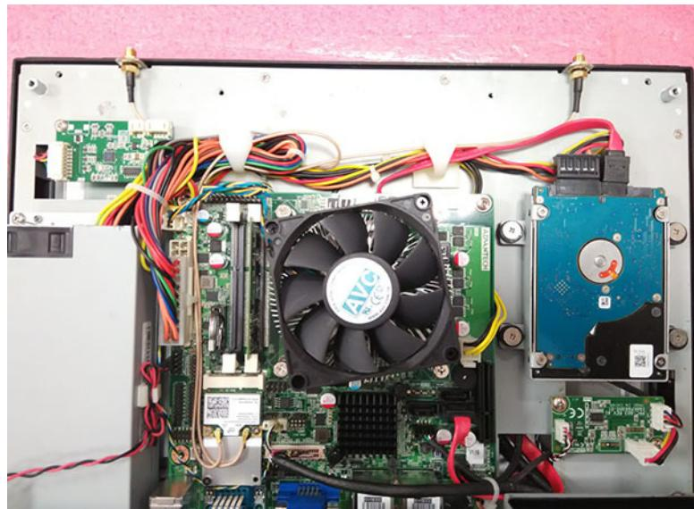
**Figure 2.20 Attaching Wireless Card**
