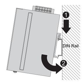
Figure 2-1. Installing the DIN-Rail Mounting Kit
