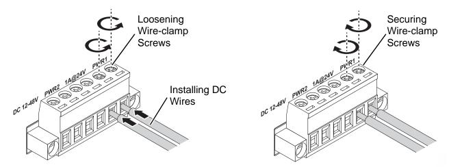
Figure 2-17. Installing DC Wires in a Terminal Block
