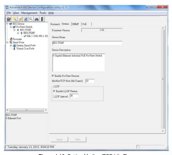
Figure 4-10. Setting Modbus/TCP Idle Time
