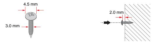
Figure 2-4. Securing Wall Mounting Screws
