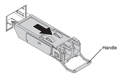
Figure 2-10. Removing an SFP Transceiver
