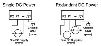
Figure 2-12. Power Wiring for EKI-5000 Series
