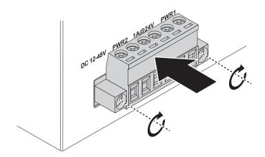
Figure 2-18. Securing a Terminal Block to a Receptor
