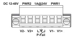
Figure 2-15. Terminal Receptor: Power Input Contacts
