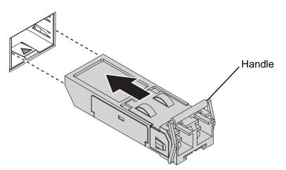
Figure 2-7. Installing an SFP Transceiver
