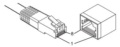
Figure 2-11. Ethernet Plug & Connector Pin Position
