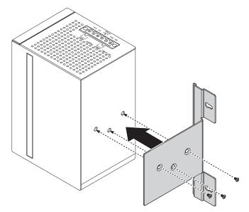
Figure 2-3. Installing Wall Mount Plates
