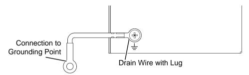
Figure 2-13. Grounding Connection
