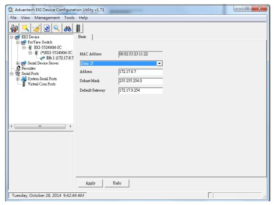
Figure 4-2. Configuring a Static IP Setting
