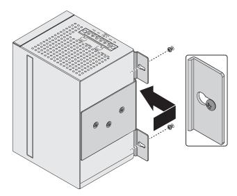
Figure 2-5. Wall Mount Installation
