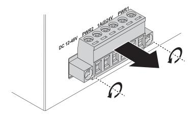
Figure 2-16. Removing a Terminal Block
