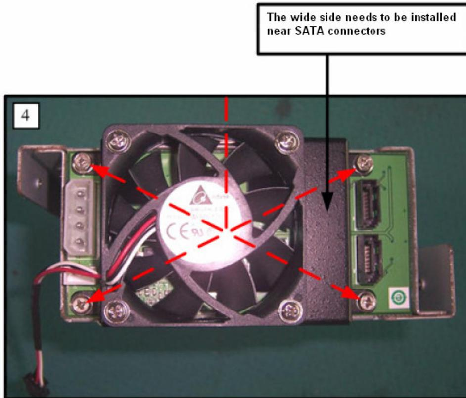
**If customer installs wrong side of FAN module, mechanism conflict issue between SATA driver bay and AIMB Main board would occur.**
