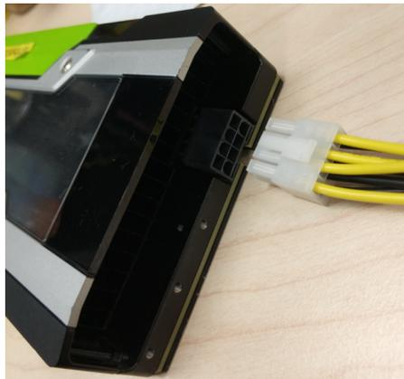
3. When installing expansion cards (e.g.:TESLA K40), use PCIe (6+2P) cable for it.
