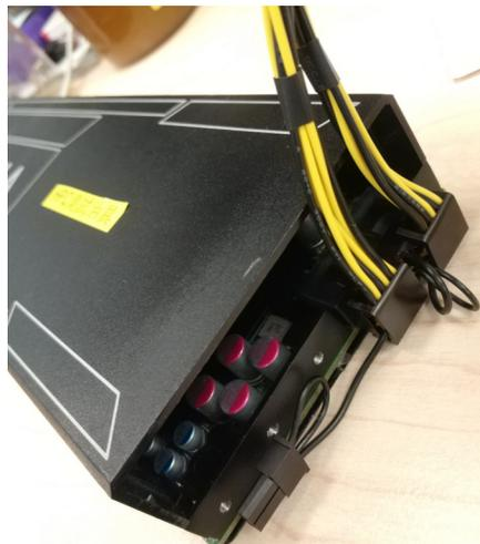
4. ONLY UL card cage can support GTX series expansion card (card length up to 280mm)
