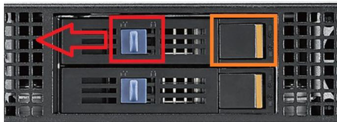
2. Place a hard drive into the drive tray and use the screws to secure the HDD, then insert the HDD tray into the chassis and press the locking lever to secure the tray.
