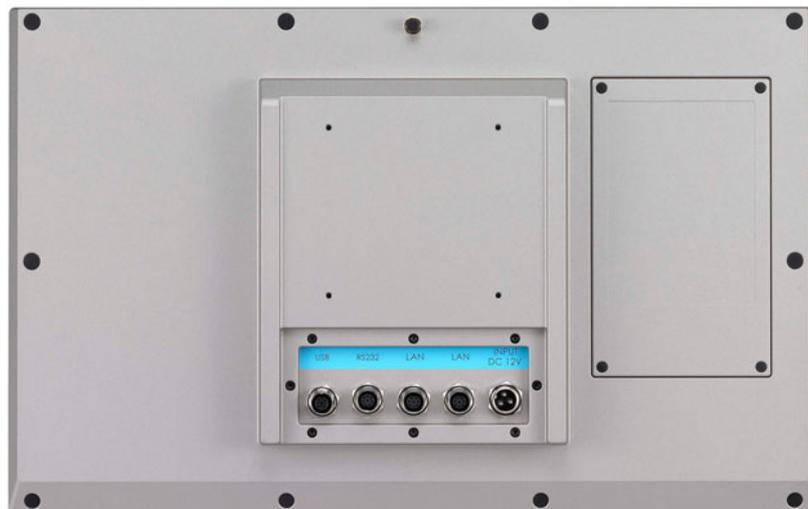
Figure 1.1 SPC-200 Rear View- I/O Port Arrangement
