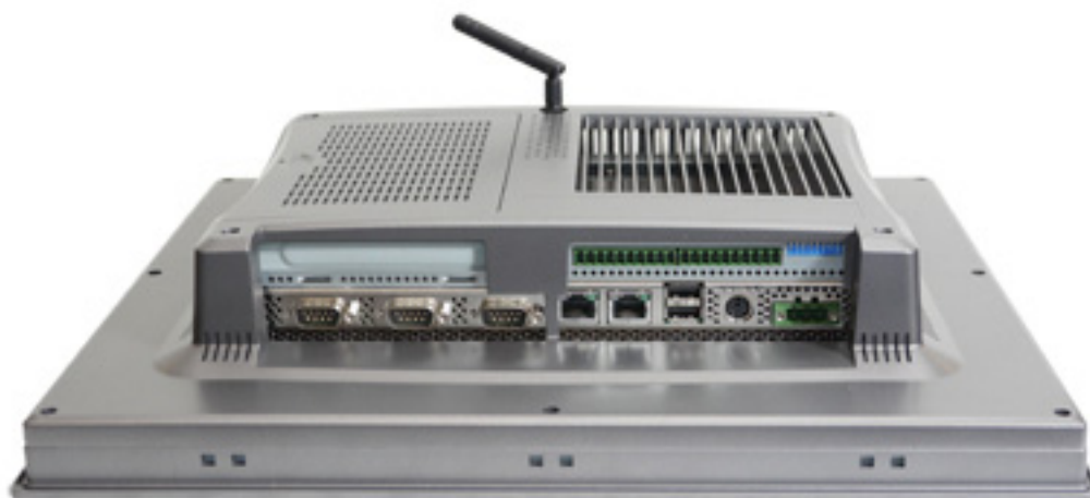
Figure 1.2 TPC-1571H/1771H - I/O Port Arrangement (Antenna is optional. Use P/N:1750000318 to order)
