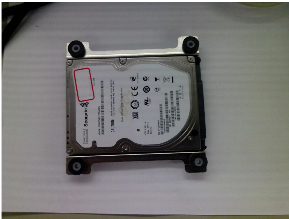
Figure C.3 Installing HDD in the holder
