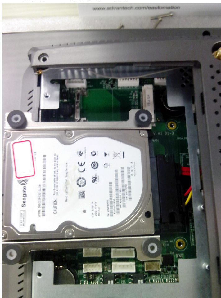
Figure C.4 Connecting the HDD cable
