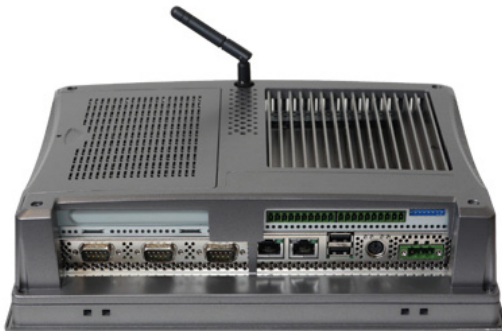
Figure 1.1 TPC-1071H/1271H - I/O Port Arrangement (Antenna is optional. Use P/N:1750000318 to order)
