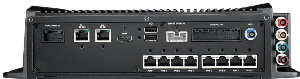
Figure 2.8 TREK-60 I/O View (with PoE)
