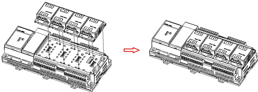
Figure 3.3 Expansion Module Installation
