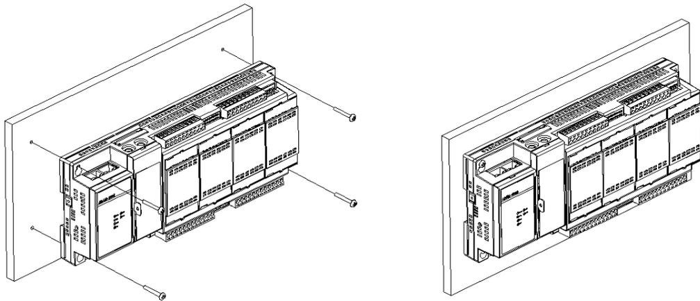
Figure 3.2 Wall-Mounted Installation
