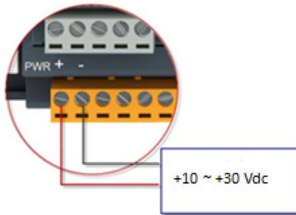
Figure 3.5 Power Supply Wiring
