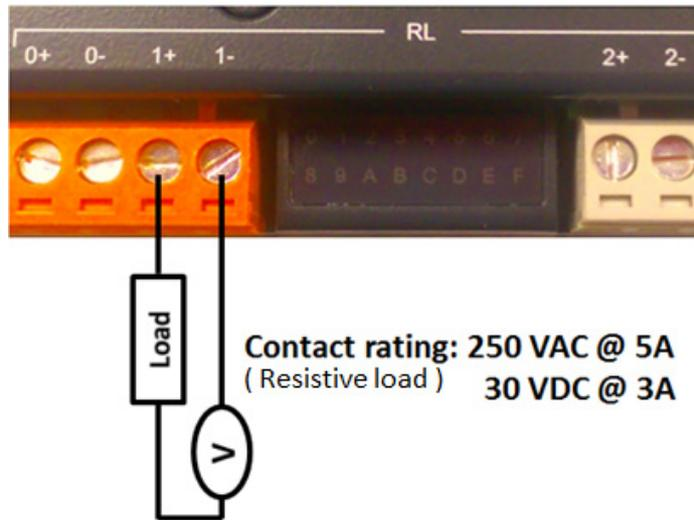
Figure 2.2 Relay Output Wiring
