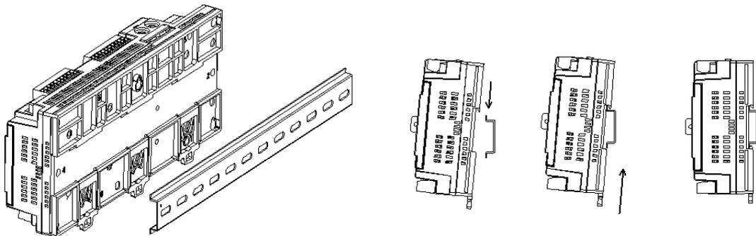
Figure 3.1 DIN-Rail Installation
