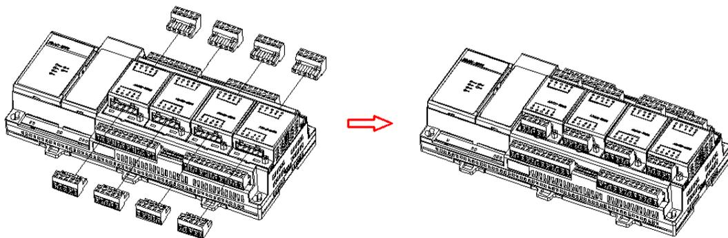
Figure 3.4 Expansion I/O Connector Installation
