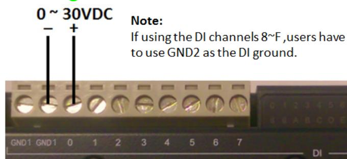
Figure 2.1 ADAM-3600-A1F Digital Input Wiring
