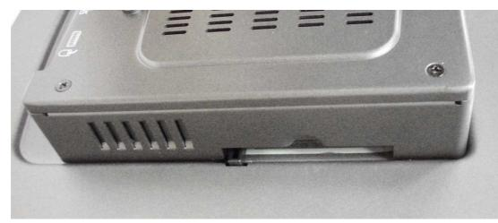
Figure 2.2 Install CFast Memory Card (Mylar in accessory box can be attached to CFast card for easy extraction)
