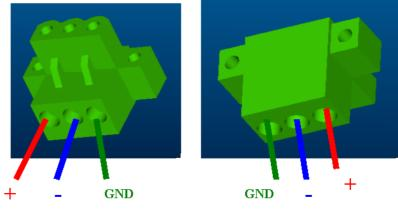
Figure 2.3 Power Connector and Power Lines
