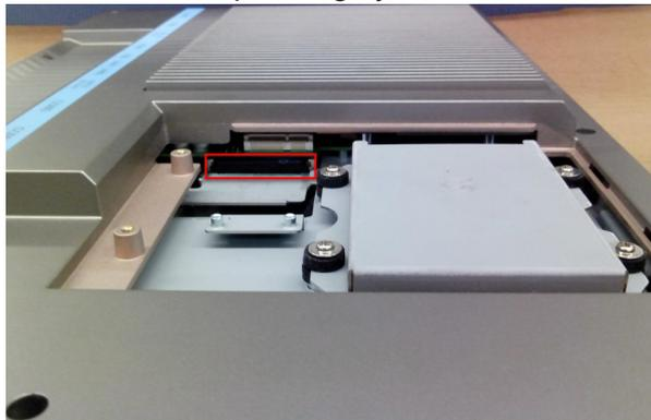
**Figure 2.2 Install CFast Memory Card**
