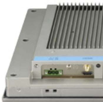
**Figure 2.4 Power Receptor**
