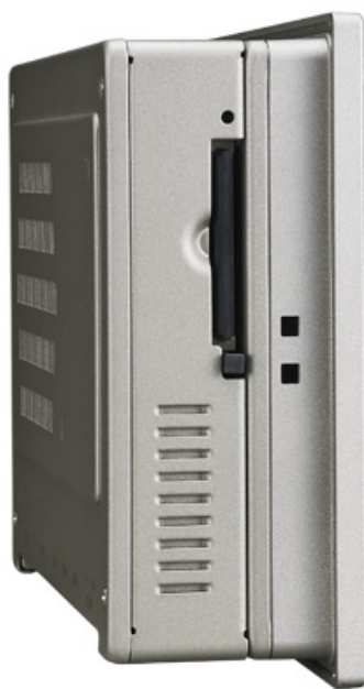
Figure 2.2 Install CFast Memory Card
