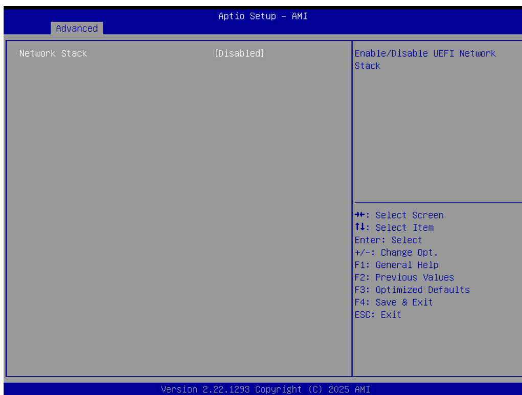
Figure A.17 Network Stack Configuration
