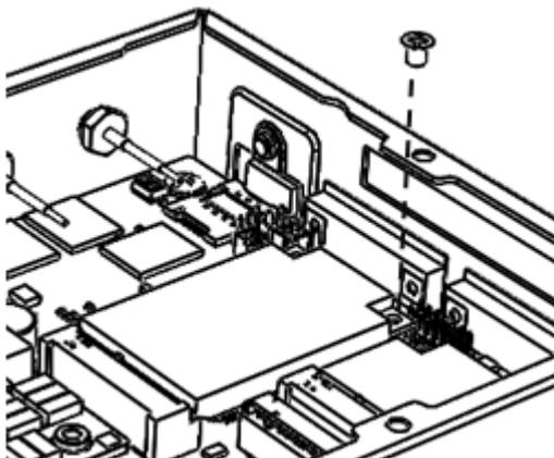
4. Assemble SMA socket to correspond SMA slot, then plug SMA cable onto wireless module.
