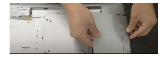
2. Press down on the cover firmly until the tabs snap into place, locking the cover securely in position. Repeat this for the bottom rear cover.
