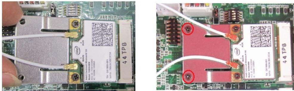
6. Cable routing of the wireless antenna is shown below.
