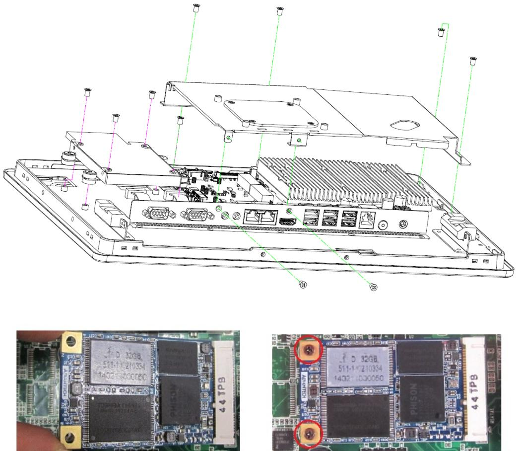
Figure 3.2 Installing the mSATA/m.2 Card
