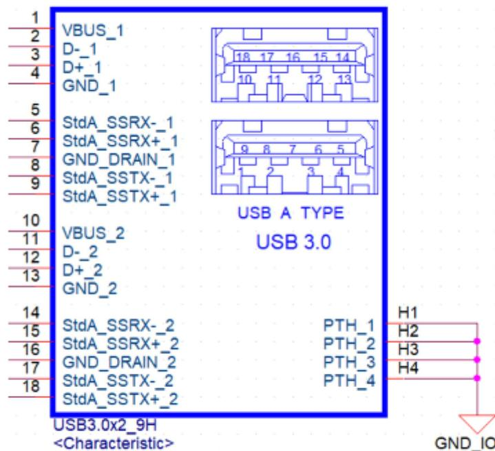
**Table A.33: CN24,CN25 (D),CN18(EF),CN20(G):External USB**
