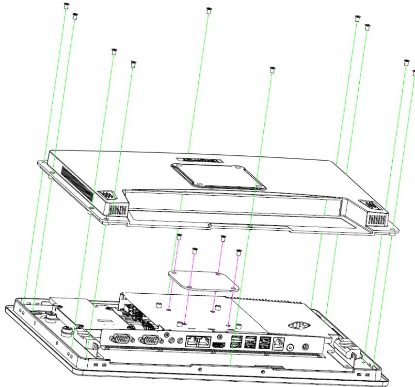
2. Remove 6 screws on the reinforced board.
