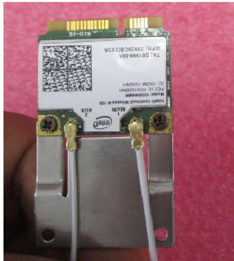
5. Install the WLAN card on M/B bottom side.
