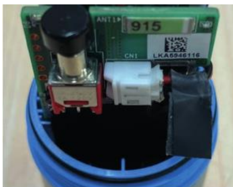
Figure 3.13 Battery Replacement Step 5
