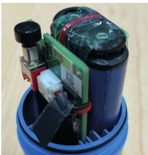
Figure 3.14 Battery Replacement Step 6
