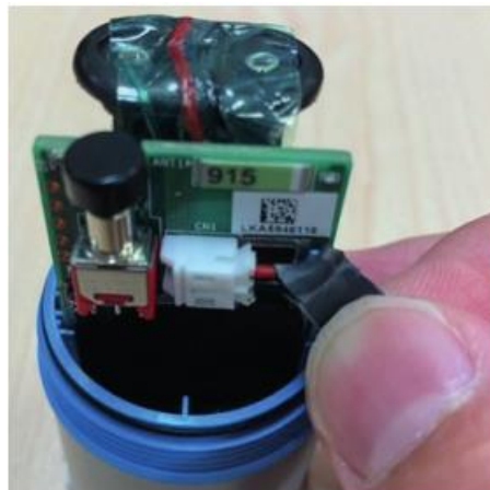
Figure 3.10 Battery Replacement Step 2
