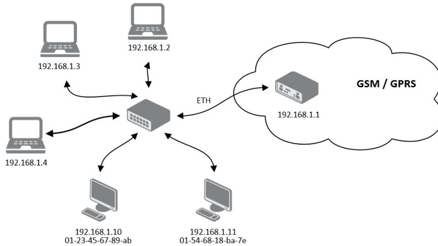
Figure 13: Example 2 – Network Topology with both Static and Dynamic DHCP Servers
