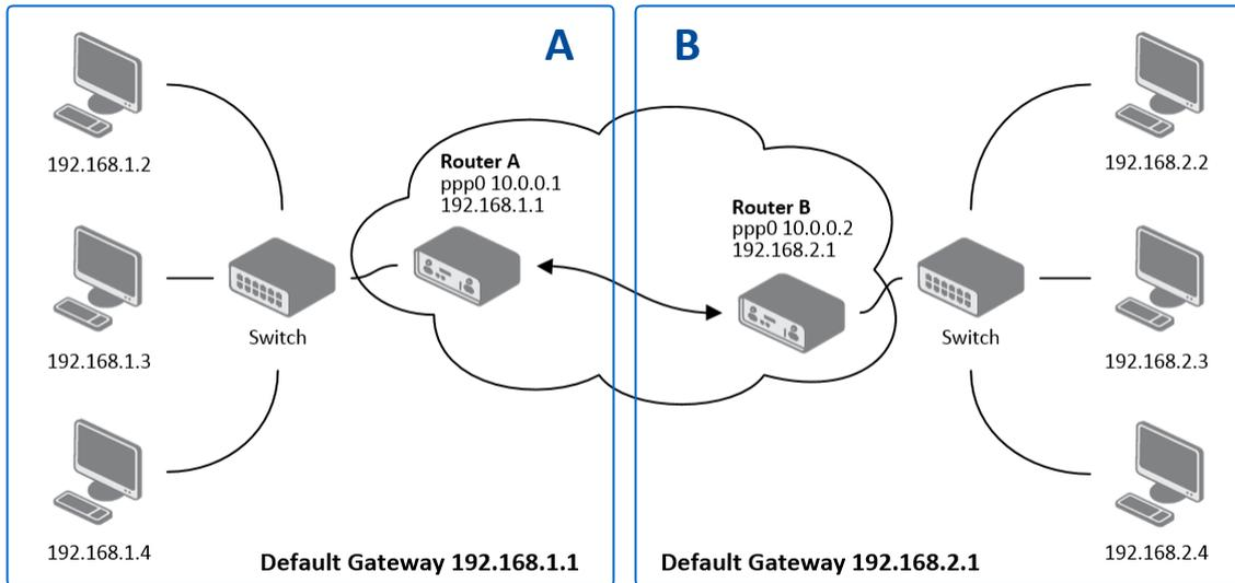
Figure 44: Topology of PPTP Tunnel Configuration Example
