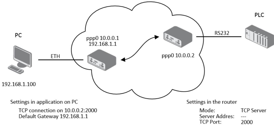
Figure 61: Example of Ethernet to serial communication
