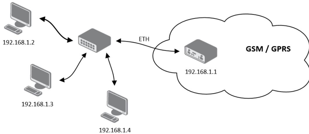
Figure 11: Example 1 – Network Topology for Dynamic DHCP Server
