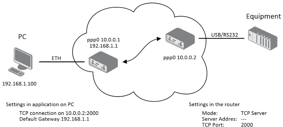
Figure 64: Example 1 – USB port configuration
