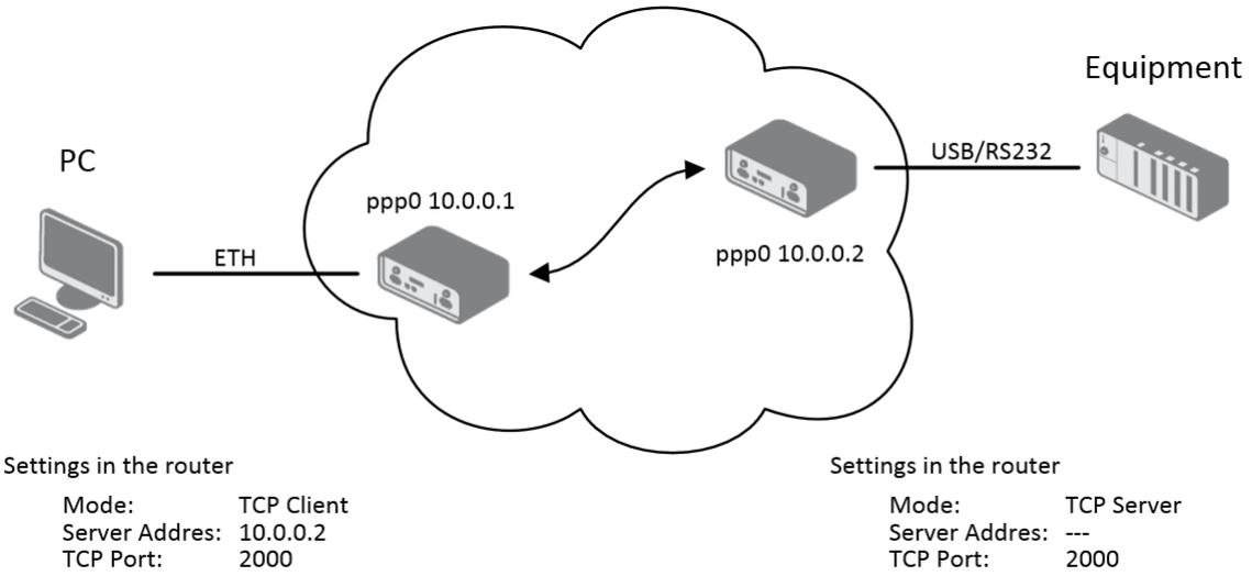
Figure 65: Example 2 – USB port configuration
