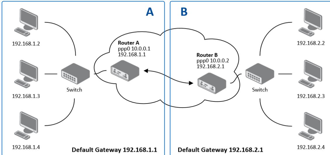
Figure 42: Topology of L2TP Tunnel Configuration Example
