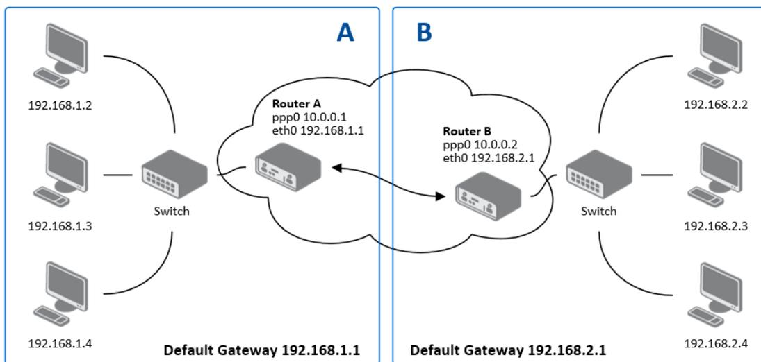
Figure 40: Topology of GRE Tunnel Configuration Example
