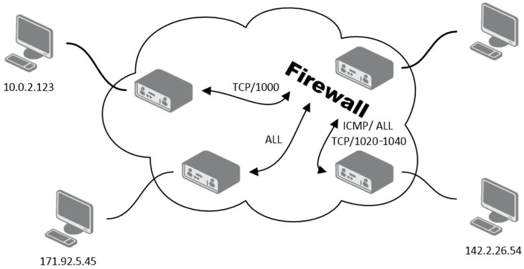
Figure 29: Topology for the Firewall Configuration Example
