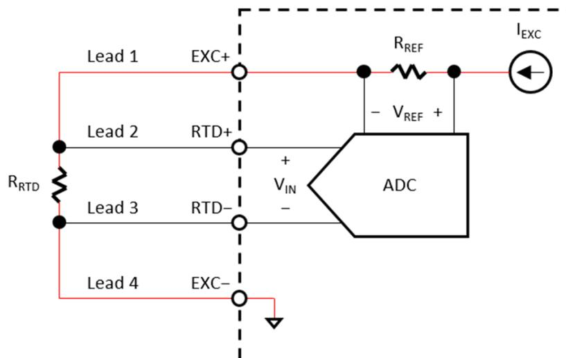
Figure 2.4 4-wire RTD input signal connection.
