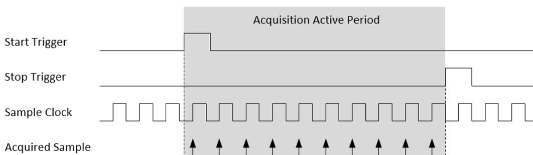
**Figure 3.3 Start and stop triggers of the analog input acquisition.**
