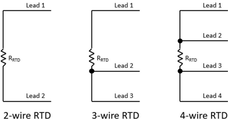
**Figure 3.5 RTD wiring configuration.**
