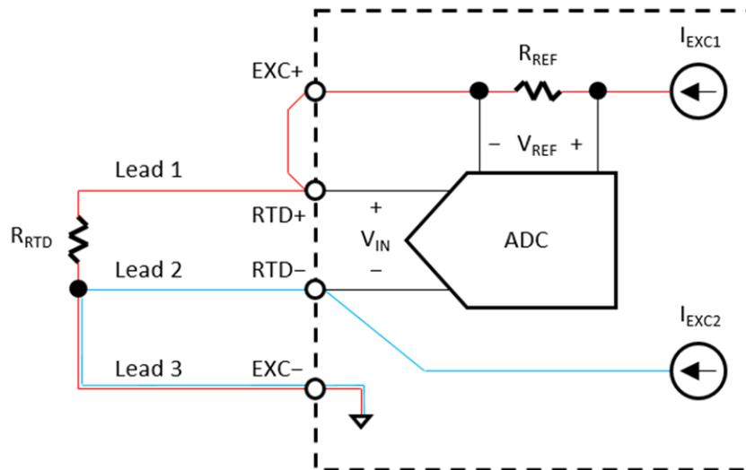
**Figure 2.3 3-wire RTD input signal connection.**
