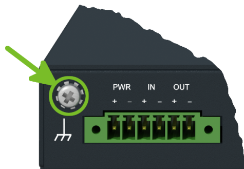
Figure 14: Position of the Grounding Screw
