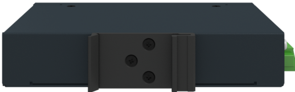
Figure 8: Position of the DIN Rail Clip
