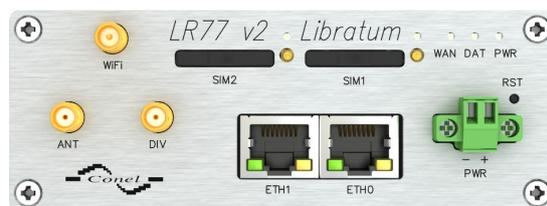
Figure 5: Front panel LR77 v2L SL with WiFi
