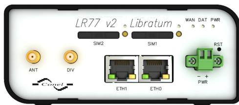
Figure 2: Front panel LR77 v2L
