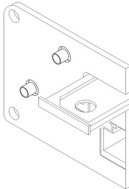
Figure 21: Ejected SIM holder
