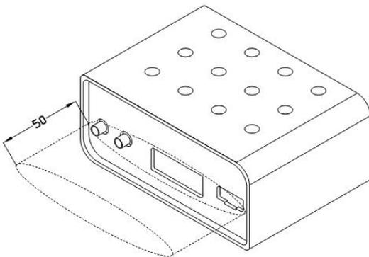
Figure 13: Space in front of connectors (plastic)
