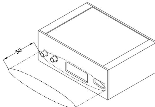
Figure 14: Space in front of connectors (metal)
