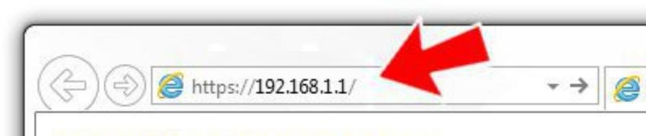
Figure 26: Entering the IP address of the router
