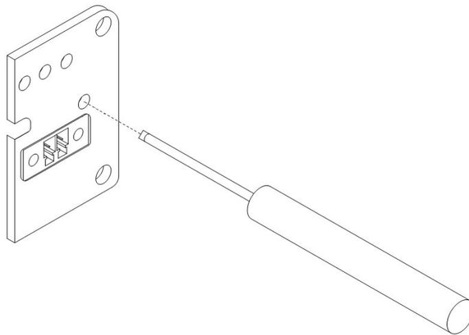
Figure 24: Router reset
