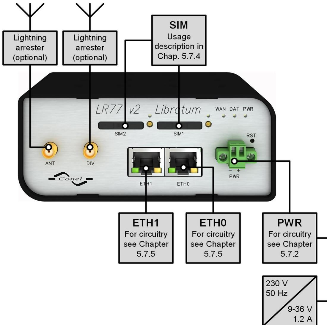
Figure 25: Router connection
