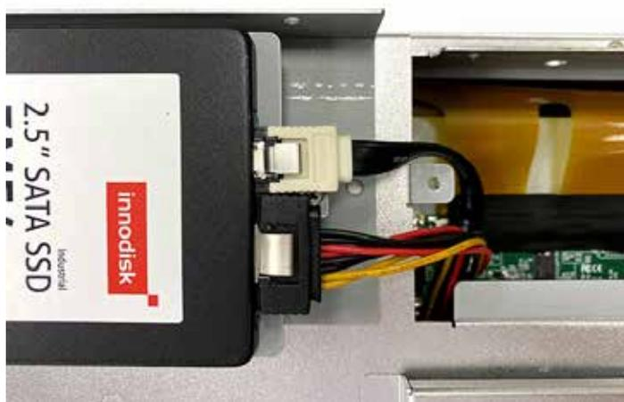
**Step 6** Put back storage cover with storage bracket to system and puck up it with 4 pcs screws.
