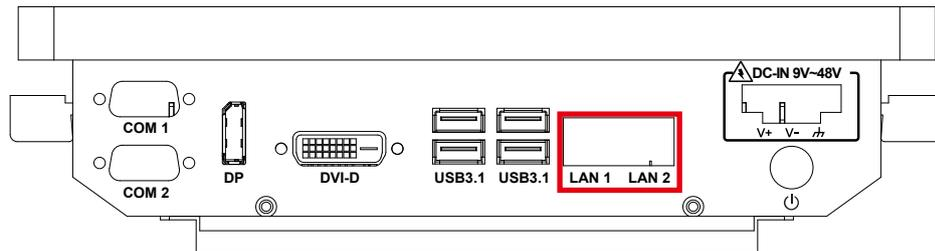
There are dual 8-pin RJ-45 jacks supporting 10/100/1000 Mbps Ethernet connections in the front side. LAN 1 is powered by Intel® i219 Ethernet Phy; LAN 2 is powered by Intel® I210 Ethernet engine. When both of LANs work in normal status, iAMT function is enabled. Using suitable RJ-45 cable, you can connect the system to a computer, or to any other devices with Ethernet connection, for example, a hub or a switch. Moreover, both of LANs support Wake on LAN and Pre-boot functions.
