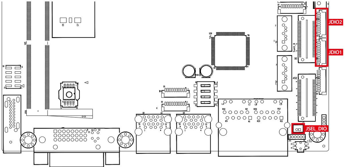
There is a 16-bit GPIO connector in the Top side. Each GPIO channel can be configuration GPI or GPO.
