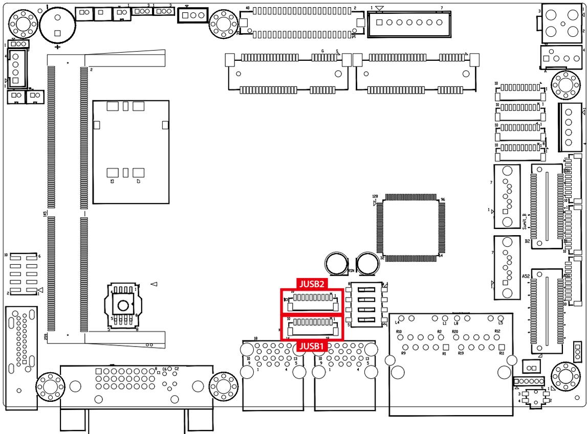
The EMBC-3000 main board provides maxima eight expansion USB ports. The USB interface supports 480Mbps transfer rate which comply with high speed USB specification Rev. 2.0.
