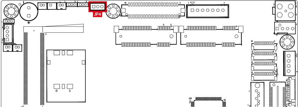
JP4 provides LVDS voltage selection function, Closing Pin 1 and Pin 2 is for 3.3V LVDS power input; closing Pin 2 and Pin 3 is for 5V LVDS power input.
