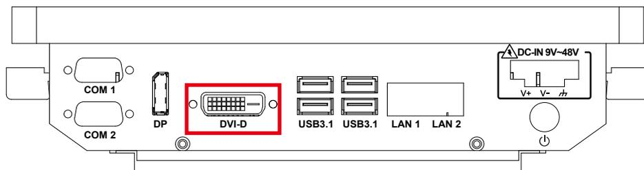
The DVI output mode supports up to 1920 x 1080 resolution. The DVI is automatically selected according to the display device connected. You will need a DVI-D cable when connecting to a display device.
