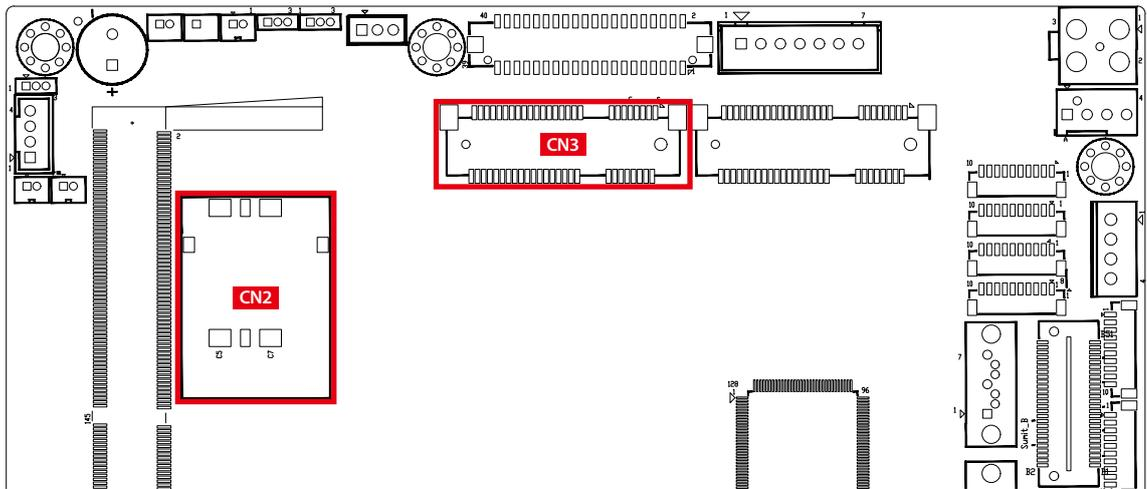
Note : The SIM card socket (CN2) do not support hot-plug. Please make sure to unplug the system power before inserting the SIM card.
