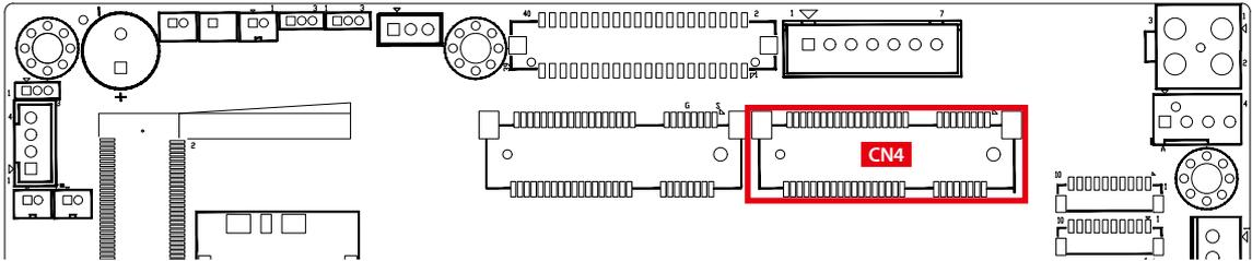
Both mSATA and Mini PCIe share the same form factor and similar electrical pinout assignments on their connectors. There was no clear mechanism to distinguish if a mSATA drive or a Mini PCIe device is plugged into the socket until recently that SATA I/O issued an ECN change (ECN #045) to redefine pin43 on mSATA connector as "no connect" instead of "return current path" (or GND).
