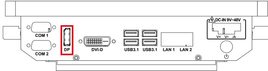
DisplayPort connection supports up to 4096 x 2304 resolution at 60Hz.
