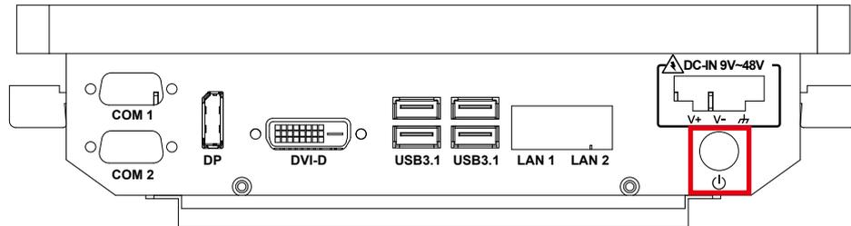
The power button is a non-latched switch. In case of system halts, you can press and hold the power button for 4 seconds to compulsorily shut down the system. Please note that a 4 seconds interval is kept by the system between two on/off operations (i.e. once turning off the system, you shall wait for 4 seconds to initiate another power-on operation).
