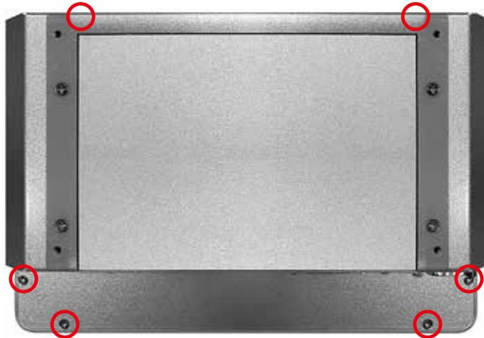
**Step 2** Remove 4pcs M3x4 screws of SSD/HDD Tray from back cover.
