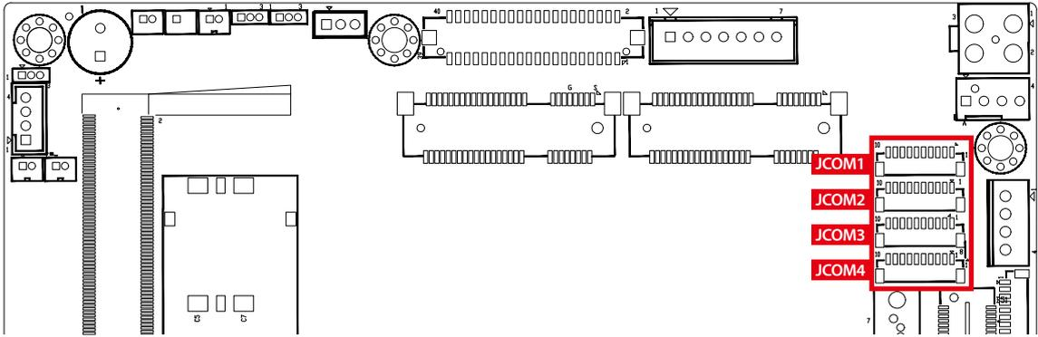
Serial port 1 to 4 (JCOM 1 to 4) can be configured for RS-232, RS-422, or RS-485 with auto flow control communication. The default definition of COM 1 to 4 is RS-232, if you want to change to RS-422 or RS-485, you can find the setting in BIOS.
