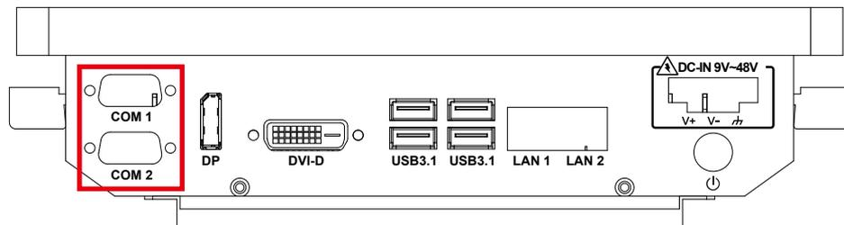
Serial port can be configured for RS-232, RS-422, or RS-485 with auto flow control communication. The default definition is RS-232, but if you want to change to RS-422 or RS-485, you can find the settings in BIOS.
