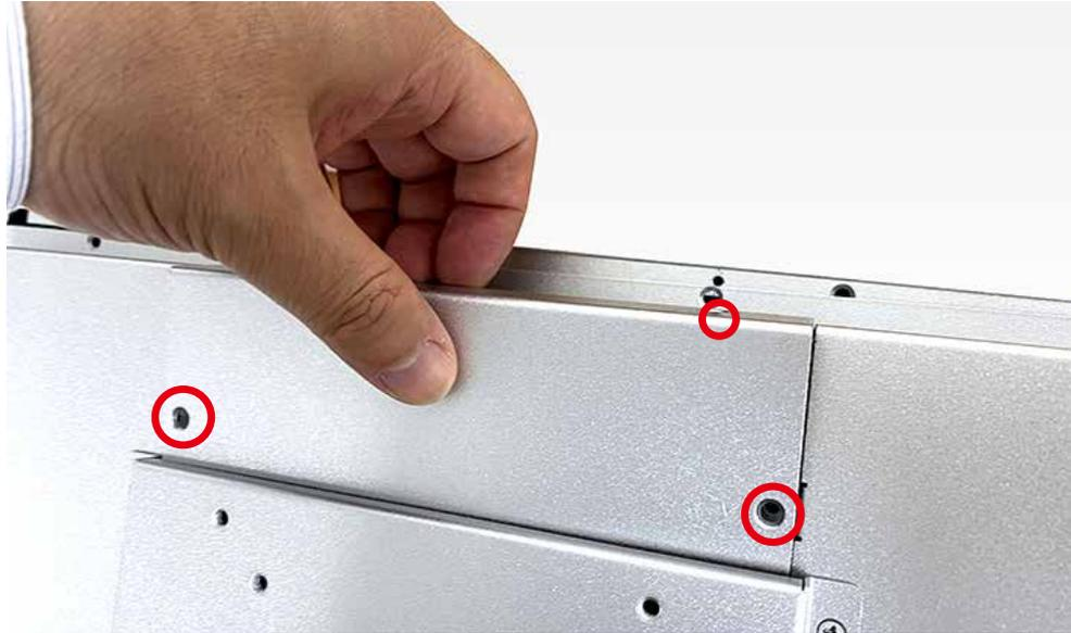
**Step 2** Loosen 2pcs screws from SSD/HDD bracket.
