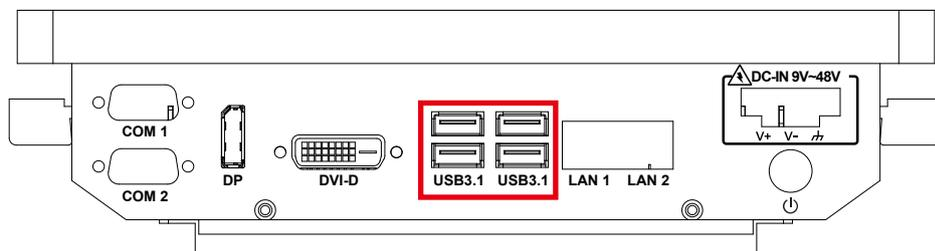
There are 4 USB 3.1 connections available supporting up to 10GB per second data rate on MTC-7000 series panel pc. It also compliant with the requirements of Super Speed (SS), high speed (HS), full speed (FS) and low speed (LS).
