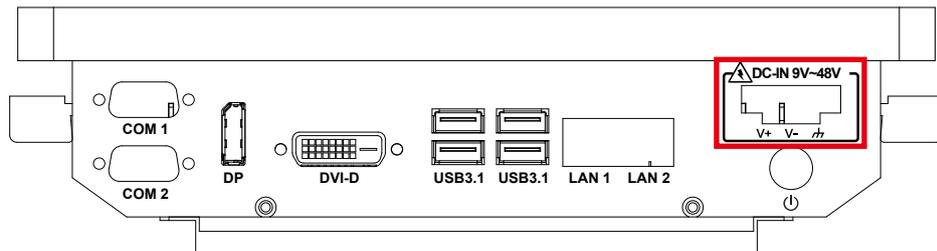
MTC-7000 supports 9V to 48V DC power input.
