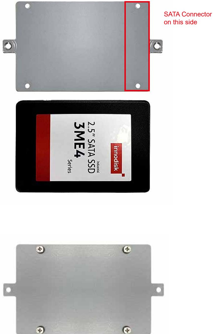
**Step 4** Lock up HDD bracket on HDD cover with 2 pcs screws.
