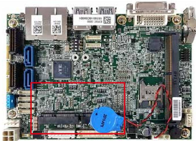
**Step 3** Install Mini PCIe card into the Mini PCIe slot.
