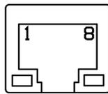
Figure 21: Ethernet connector
