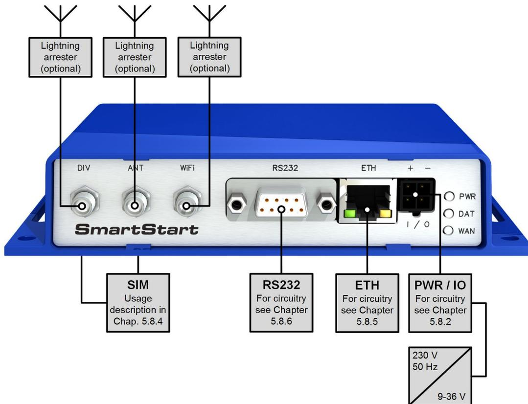
Figure 25: Router connection
