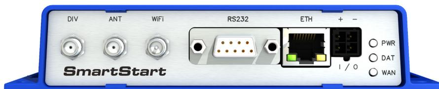
Figure 15: SmartStart front panel
